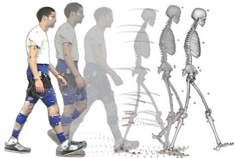
Figure 2.8: Illustration of inverse kinematics, showing the alignment of experimental marker data with a musculoskeletal model during walking[39].
