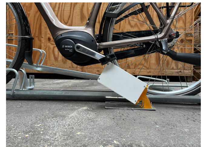
Figure 5.36: Lowered flexjoint prototype stuck under pedal during testing
