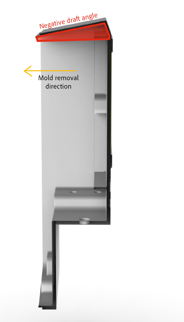
Figure 5.20: Negative draft angle in current UP-Charge design
