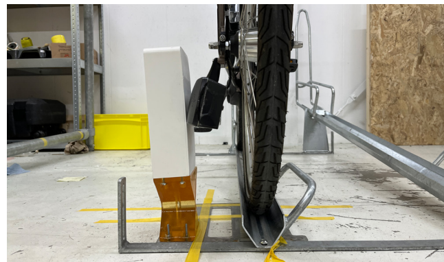
Figure 5.33: Prototype kickstand alignment & sideways flexing
