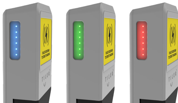
Figure 5.9: Different LED status indicators. Blue = Charging, Green = Fully charged, Red = Error
