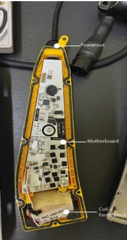
Figure 2.4: Inside of the TILER Charging Kickstand
