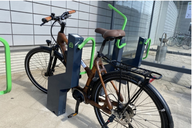
Figure 2.13: Bikeep bike locking station with integrated power outlet SOURCE: Bikeep
