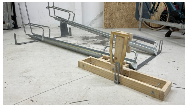
Figure 3.24: Pedal collision prototype on bike rack
