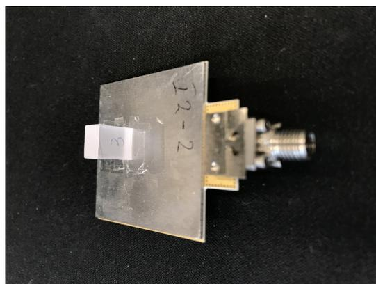
Figure 5.4: RDRA prototype for measurement
