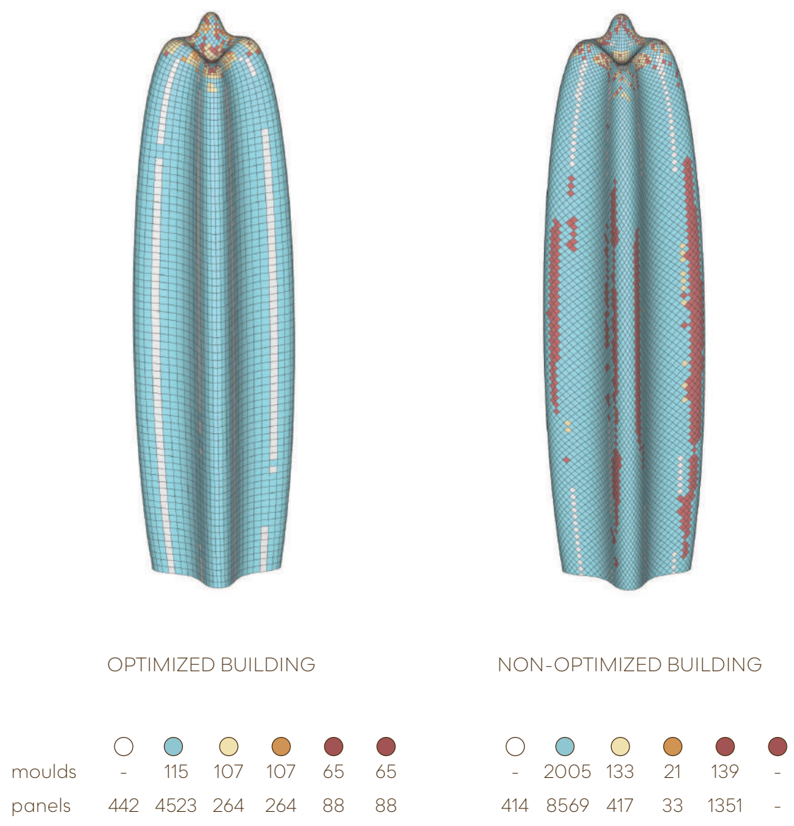
Figure 30. Comparison between an optimized and non-optimized panelization Source: Eigensatz (2010)
