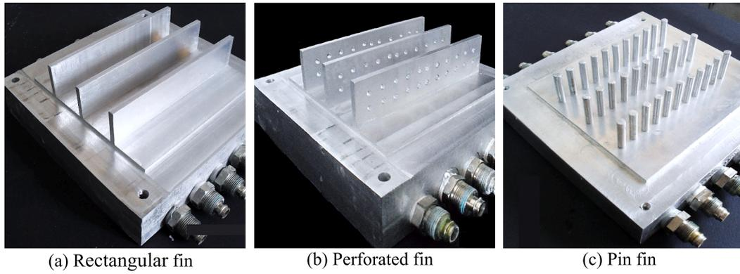
Fig. 3. The photograph of the fabricated storage tanks.
