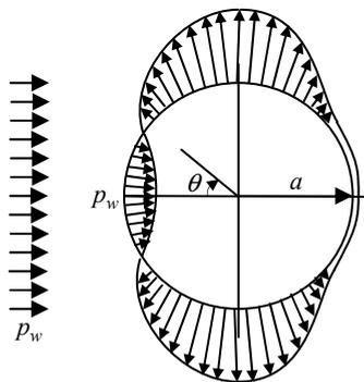
Figure 2. Typical distribution of the wind pressure
