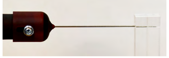
Figure 35: Biopsy needle inside the perspex duct.
