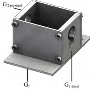
Figure 32: Positioning box ( G ), consisting of two T-profiles ( G_1 ) and two blocks ( G_2 ).
