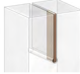
Figure 36: Mimicking the ductal lesion, using a perspex block with a key hole, to fit the gelatin sheet and to mimic the ductal tract.
