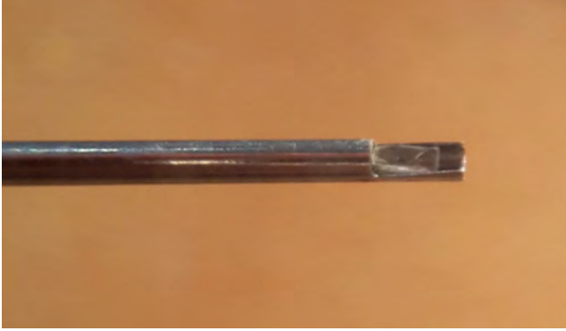
Figure 49: Tissue sample caught in the Straight knives after debulking. This example shows the ability to perform a cut.
