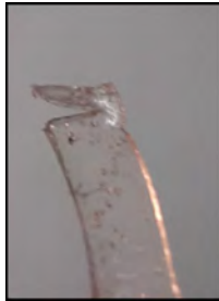
Figure 40: Failure to cut the gelatin when the Beveled knives are used.
