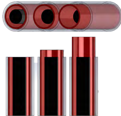
Figure 9: Push concept: The instrument containing a outer tube (Grey), which protects the ductal wall from the sharp cutting tube (Red). The cutting tube is advanced rapidly when a lesion is detected.
