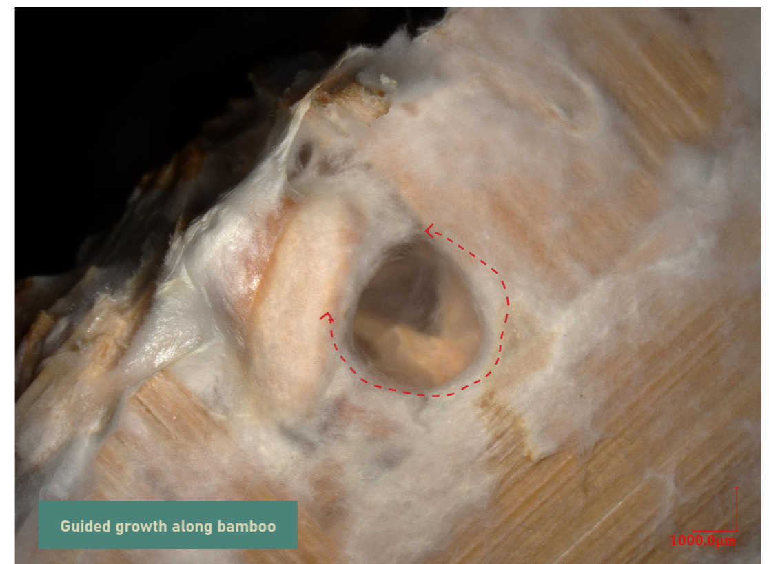
Figure 91: Growth along the bamboo woven matt surfaces (Author)
