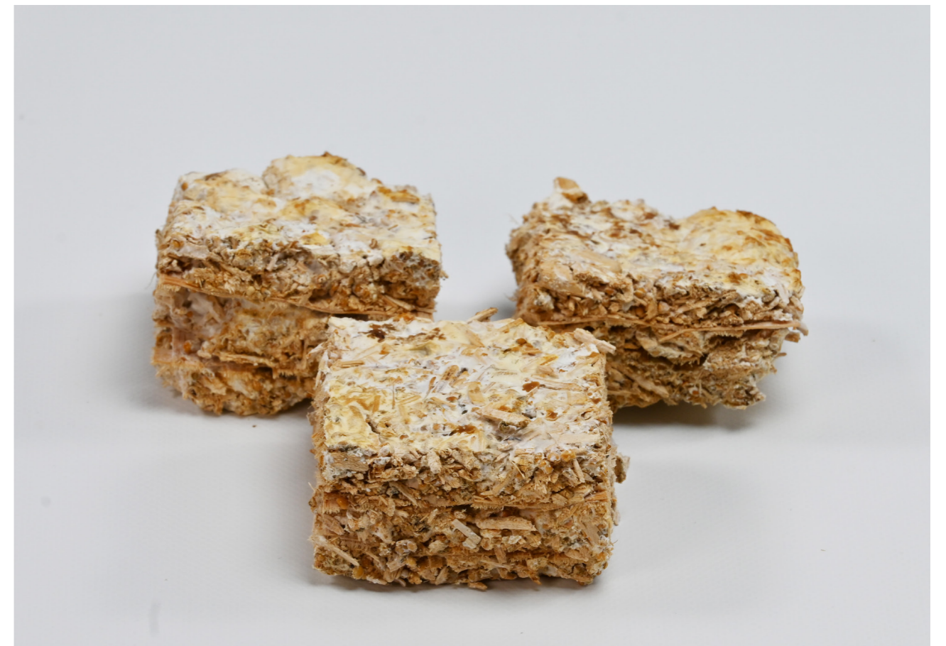
Figure 78: Thermal deactivation for 24 hours at 40°C (Author)
