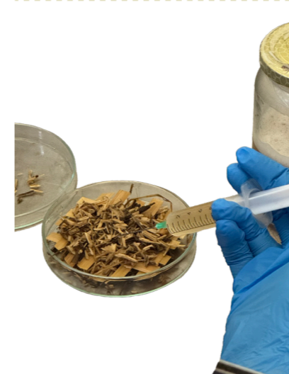
Figure 48: Sealing the substrates (Hemp, Straw, Saw dust) and WBM followed by autoclave (Author)
