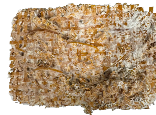
4 S.J.C.2A Completely delaminated
