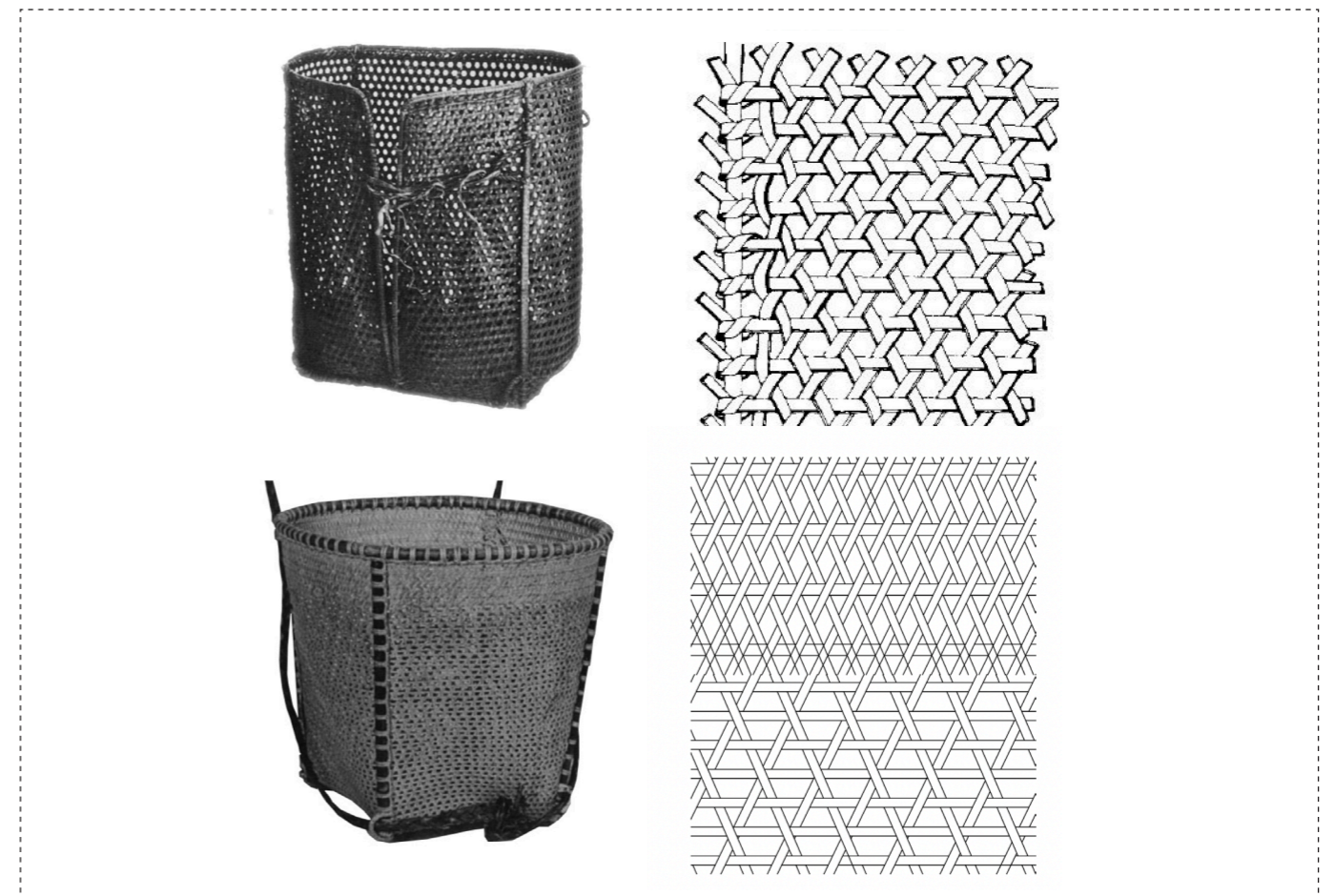
Figure 24: (top) Basket weave pattern 8mm wide, 2mm thick; (bottom) Weave pattern 3mm wide, 1.5mm thick (Source: Hebbar, 2015)
