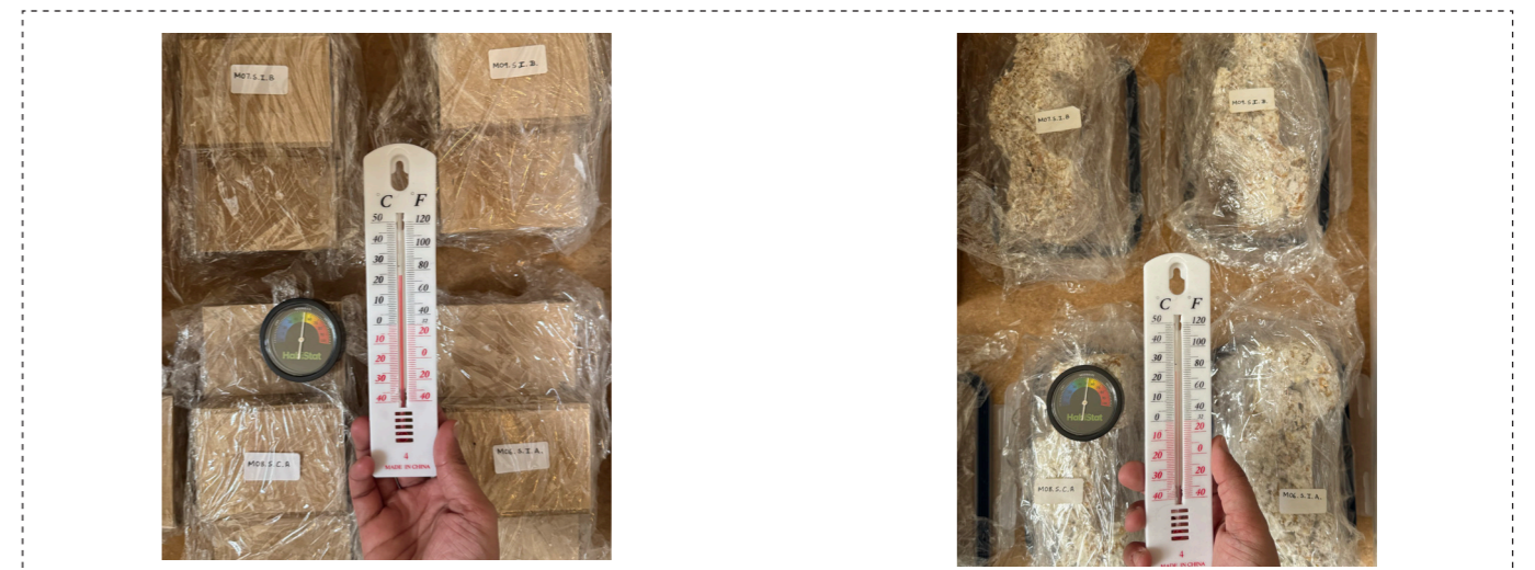
Figure 109: Stage 03: (left) Incubation, Humidity & temperature tracking; (right) After demoulding, before thermal deactivation (Author)
