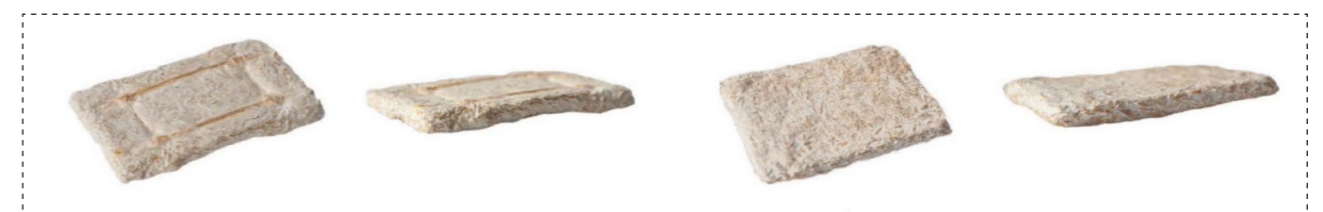
Figure 08: Results of growth on different composites. Multilayer composite (left), hemp mat sandwich (right) (Source: Nguyen et al., 2022)
