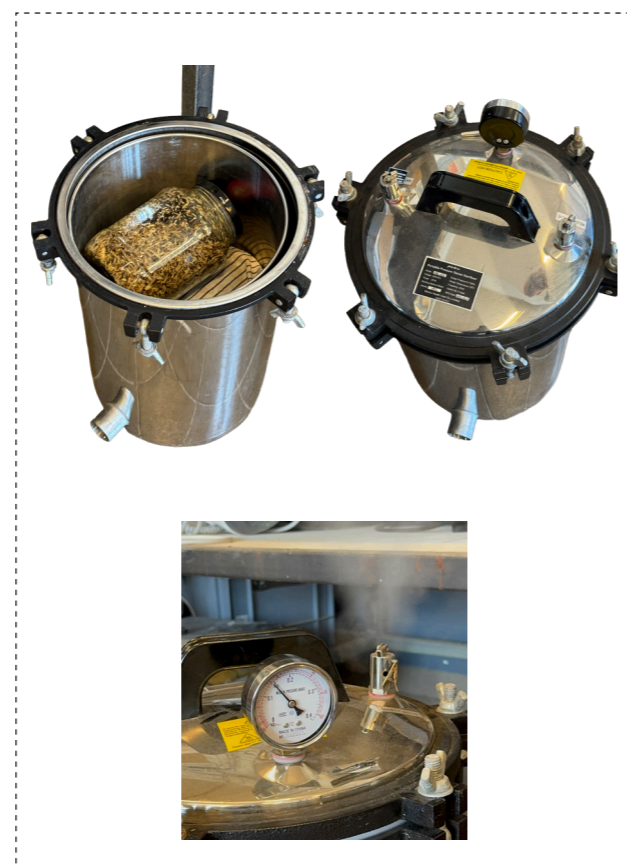
Figure 57: Medco vertical steam autoclave at 121°C for 30 minutes (Author)
