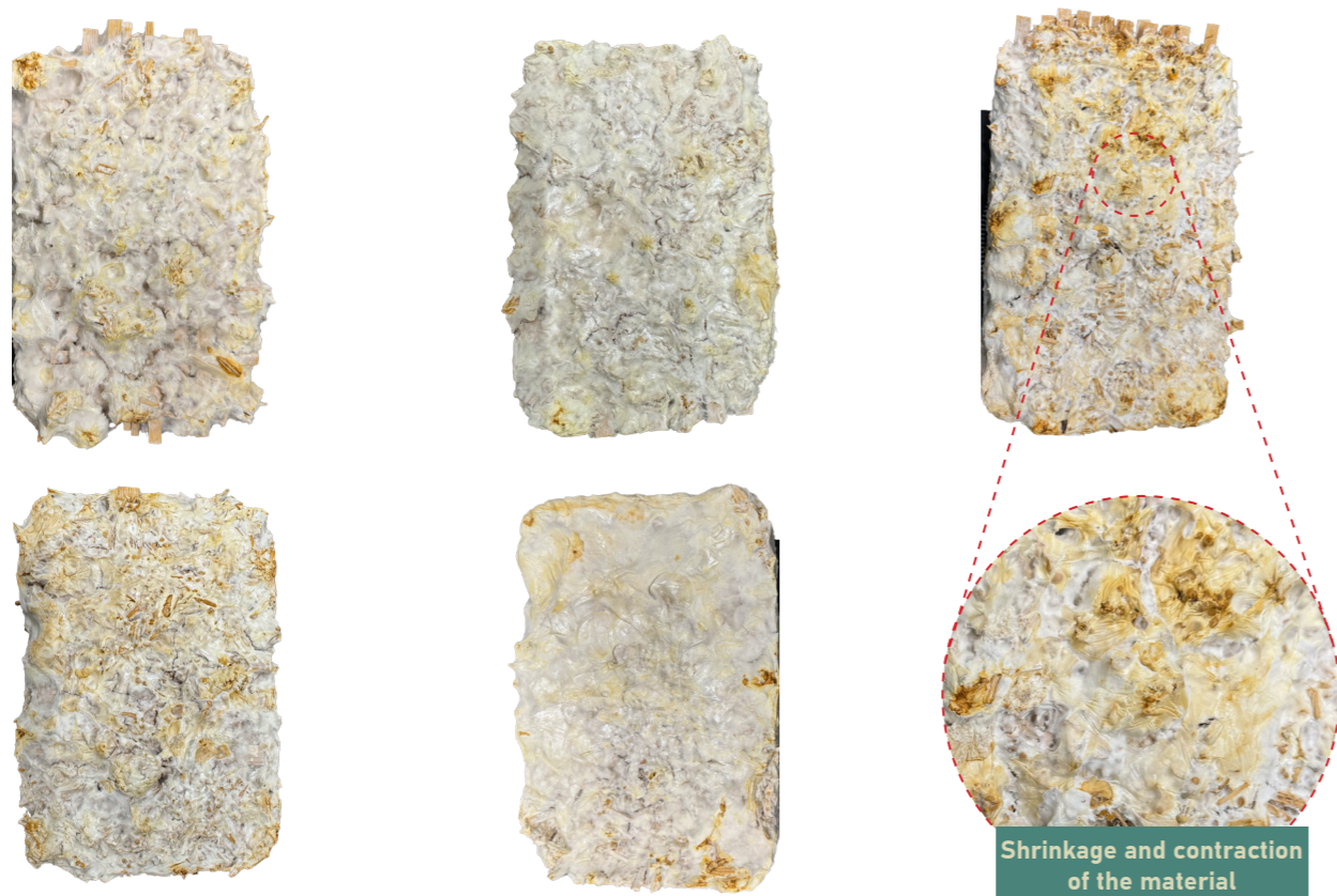
Figure 76: Thermal deactivation for 24 hours at 40°C (Author)
