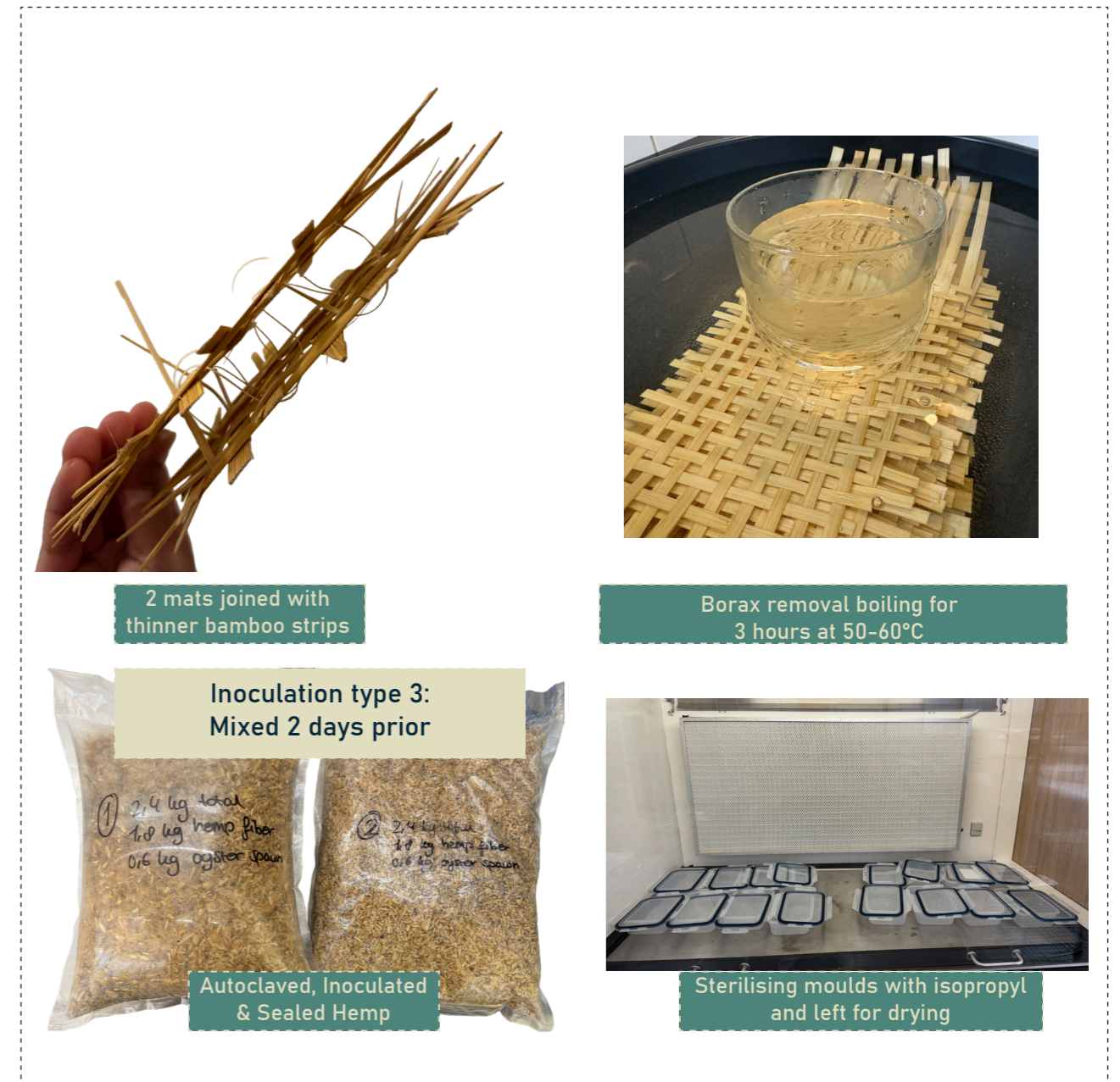
Figure 65: Stage 2A: Preparation before inoculation (Author)
