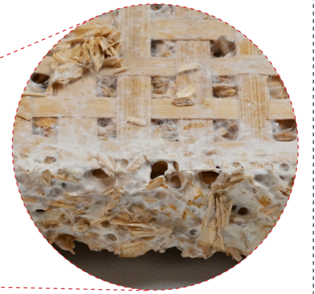
WBM and mycelial binding
