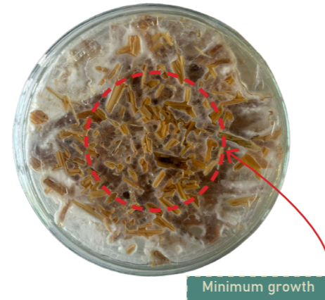
Figure 51: Minimum growth at lower side of the petri dish of the specimen LH-06 due to Liquid culture accumulation (Author)
