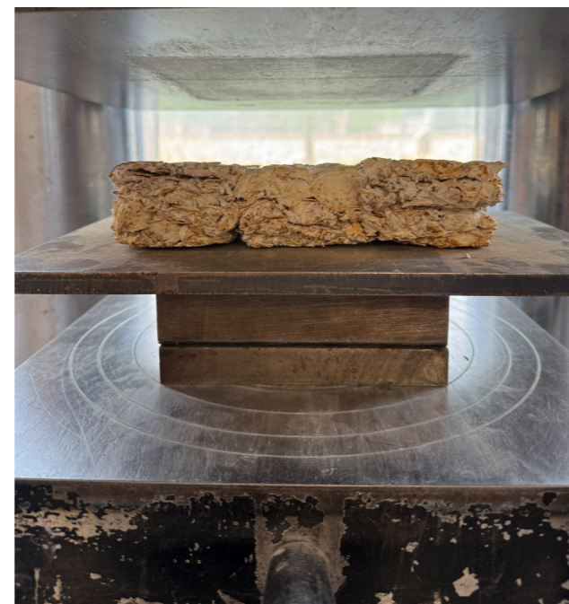
Figure 111: Specimen M07.S.I.B.(left) before and (right) after the compression test( (Source: Author)
