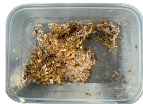
Figure 70: Stage 01: Delamination conditions after demoulding (Author)
