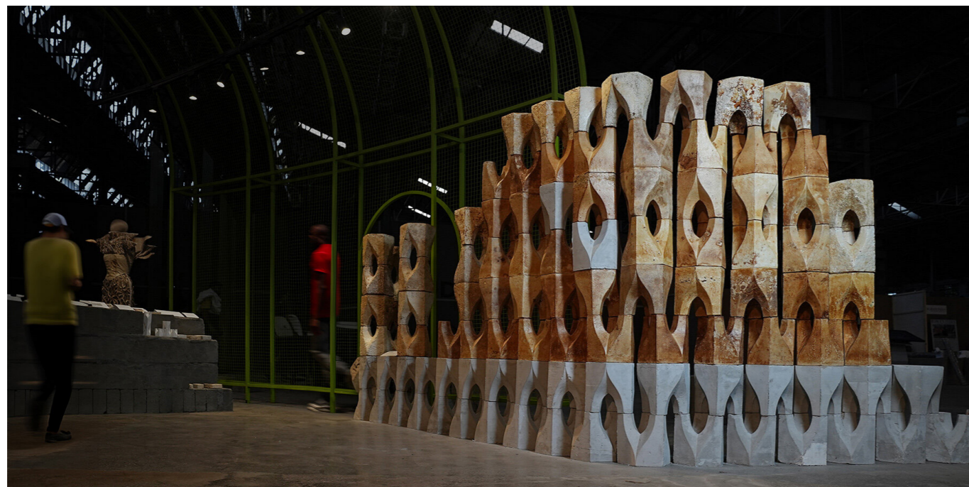
Figure 100: (top right) MycoBlox: Modular Mycelium blocks; (bottom) Wall assembly (Source: Ravenscroft, 2024)
