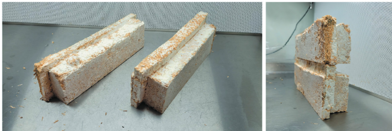
Figure 09: Two cold-pressed mixed-density module grown at 1:1 scale, approximately 400mm in width, 60mm in thickness and 100mm in height. Stacked to illustrate assembly concept (Source: Bitting et al., 2025)
