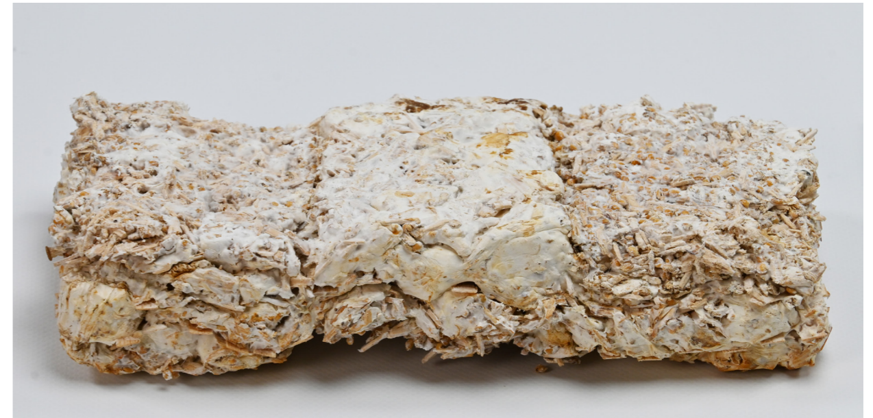
Figure 113: Stage 03: M08.S.C.A Specimen disintegration after compression test (Author)
