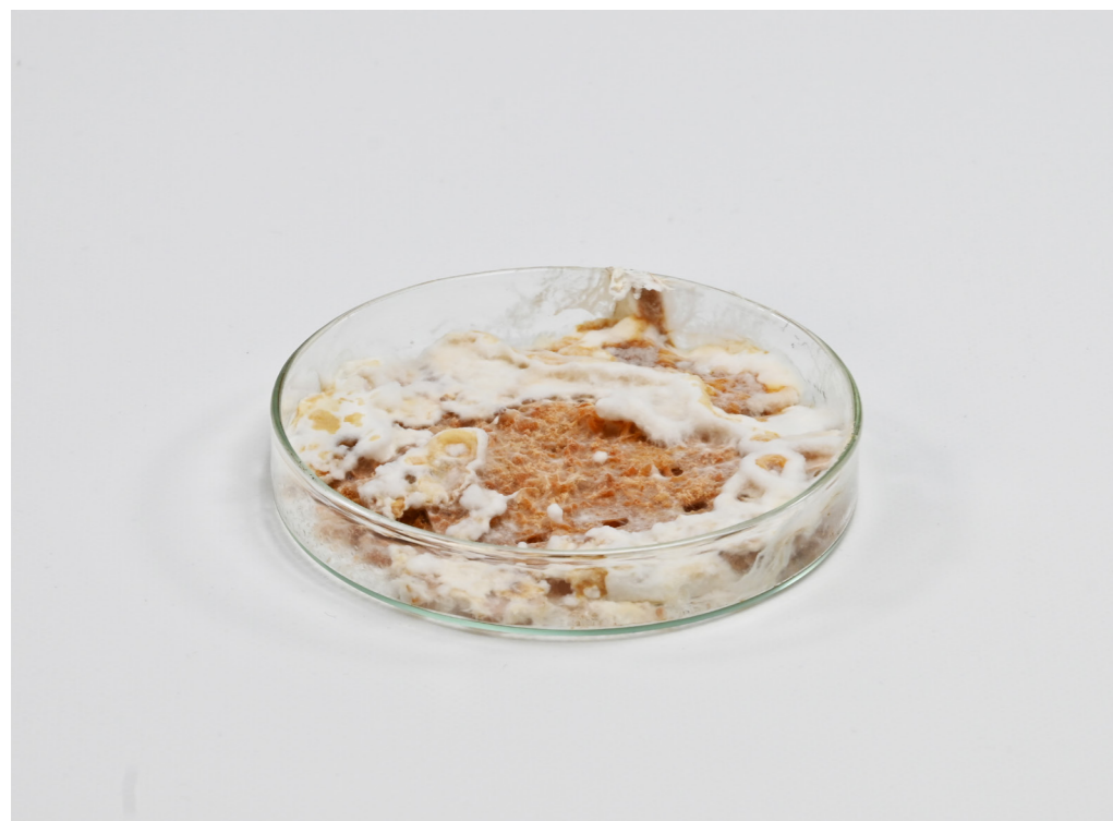
MycMax: Reinforced load-bearing MBC
