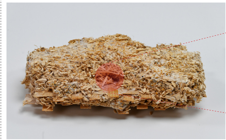
Figure 75: Specimens after Thermal deactivation from Stage 01 & 2A (Author)
