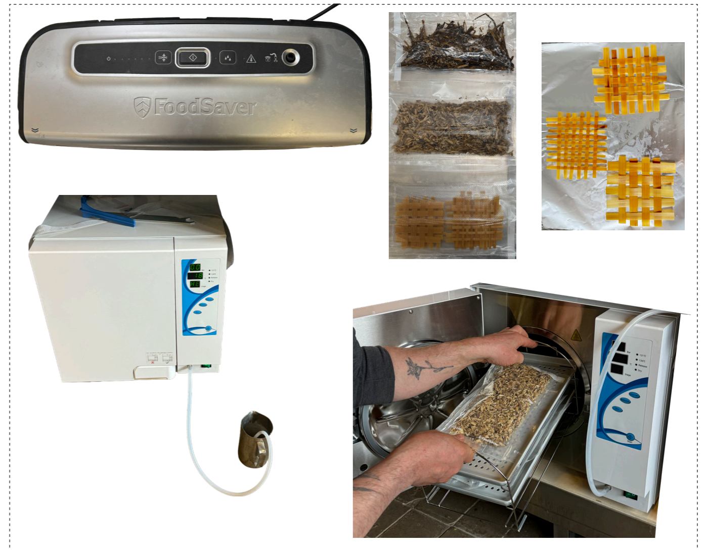
Figure 46: Sealing the substrates (Hemp, Straw, Saw dust) and WBM followed by autoclave (Author)
