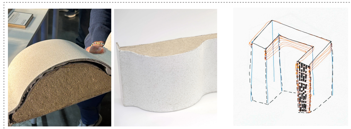
Figure 96b: (left, middle) Pre-fabricated mycelium based panels (load-bearing) (Author)
