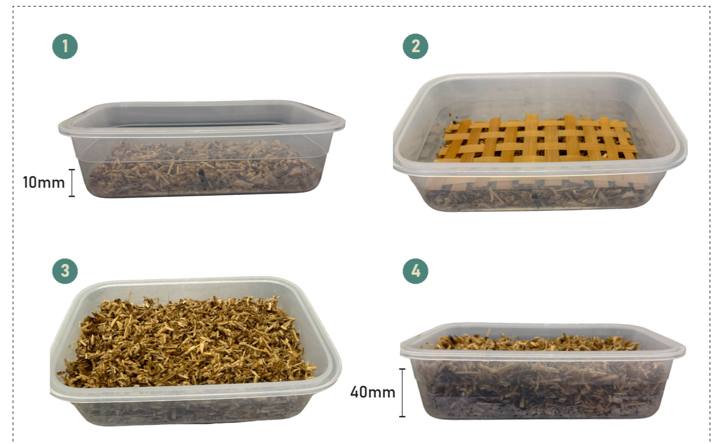
Figure 59: Assembly, (1) Mycelium inoculated hemp at 10mm (2) Placing 1 WBM large width 10mm; (3&4) Loosely packed Mycelium inoculated hemp at 10mm (Author)
