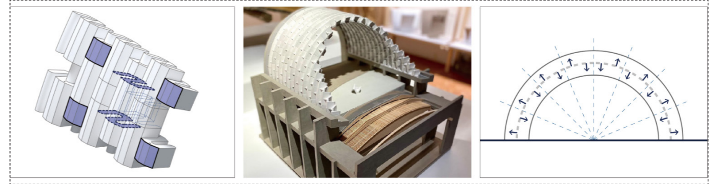
Figure 11: Proposed interlocking mechanism (left), Click brick arch (middle) and principle circular stress line (right). (Source: Tseng et al., 2024)
