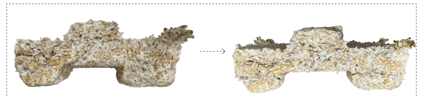
Figure 110: M07.S.I.B: (left) After demoulding, before thermal deactivation; (right) After thermal deactivation (Author)
