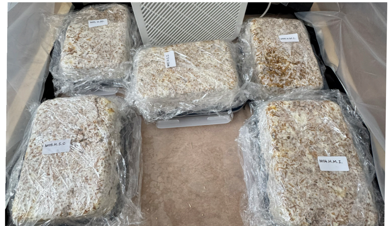
Figure 73: Stage 2B: Demoulded for mycelial skin formation before 2 days before deactivation (Author)
