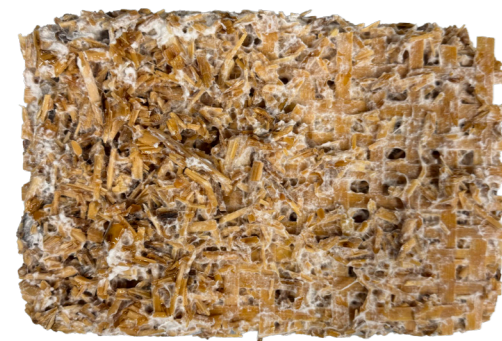
1M.He.04 Complete delamination
