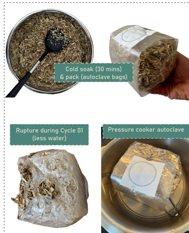
Figure 43: Hemp preparation & autoclave (Author)
