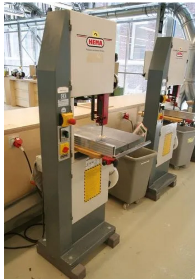
Figure 79: Hema band saw at the Model hall-wood workshop, Faculty of Architecture (Author)
