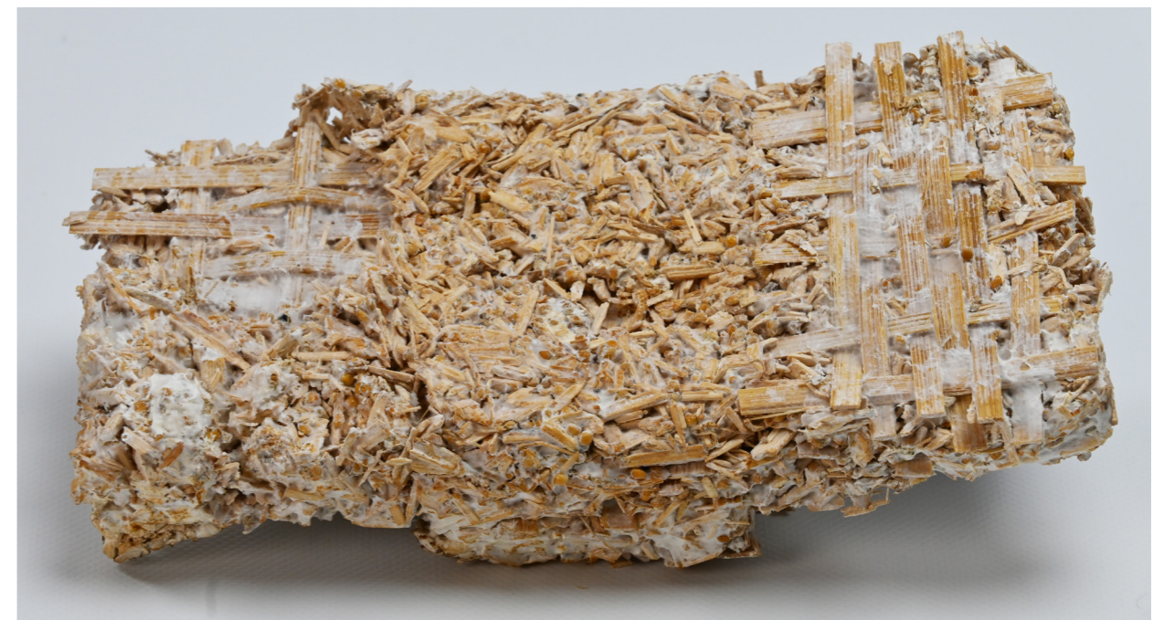
Figure 114: Stage 03: M06.S.I.A Specimen with delamination at both the legs of the specimen; After compression test (Author)
