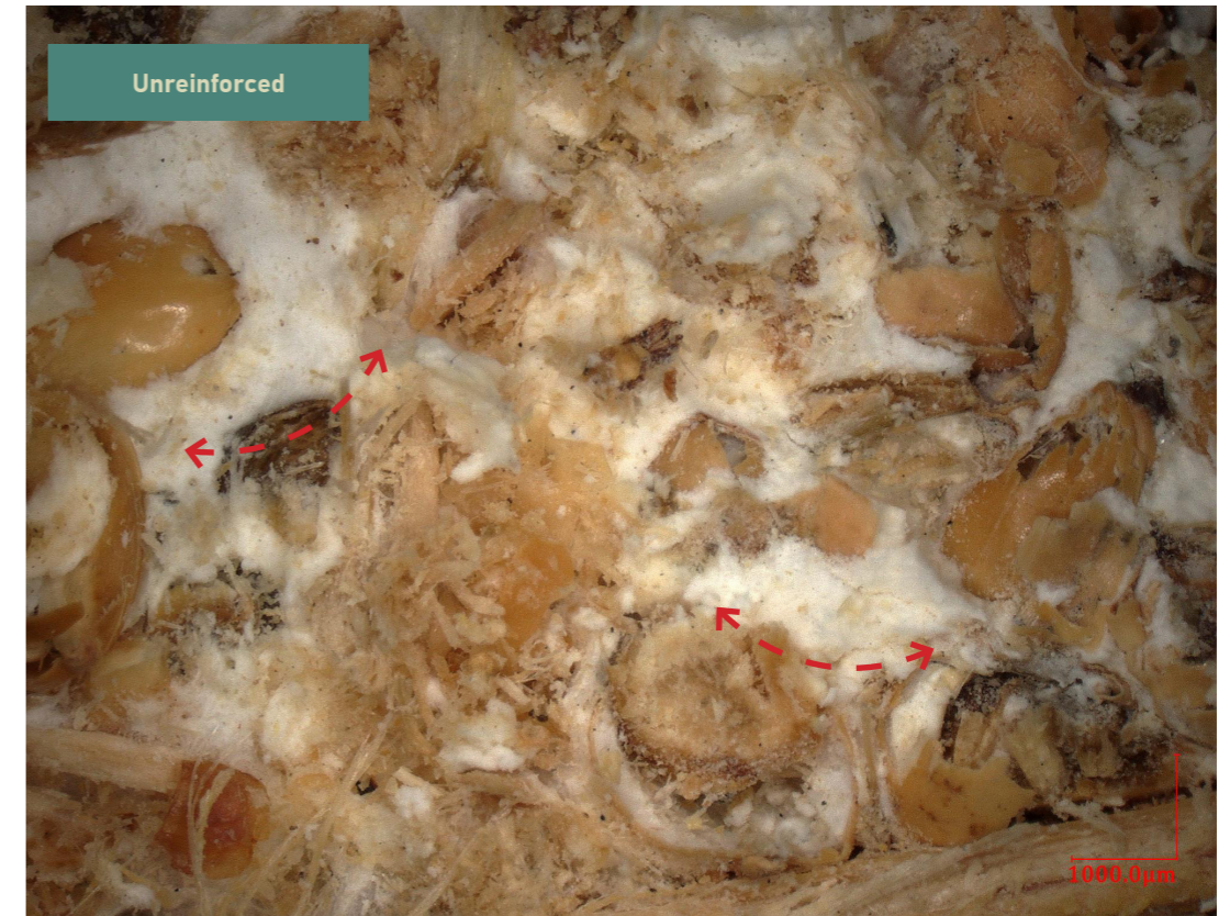
Figure 86: Growth patterns in unreinforced composite system (Author)
