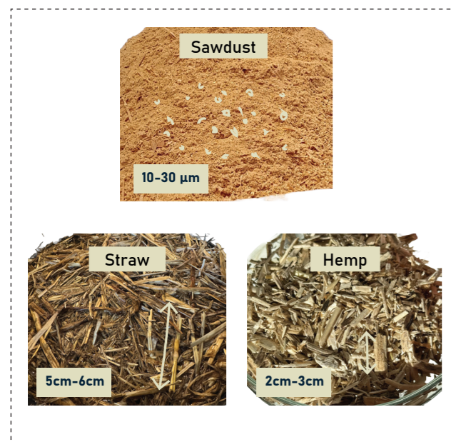
Figure 29: Particle size of each substrate (Author)
