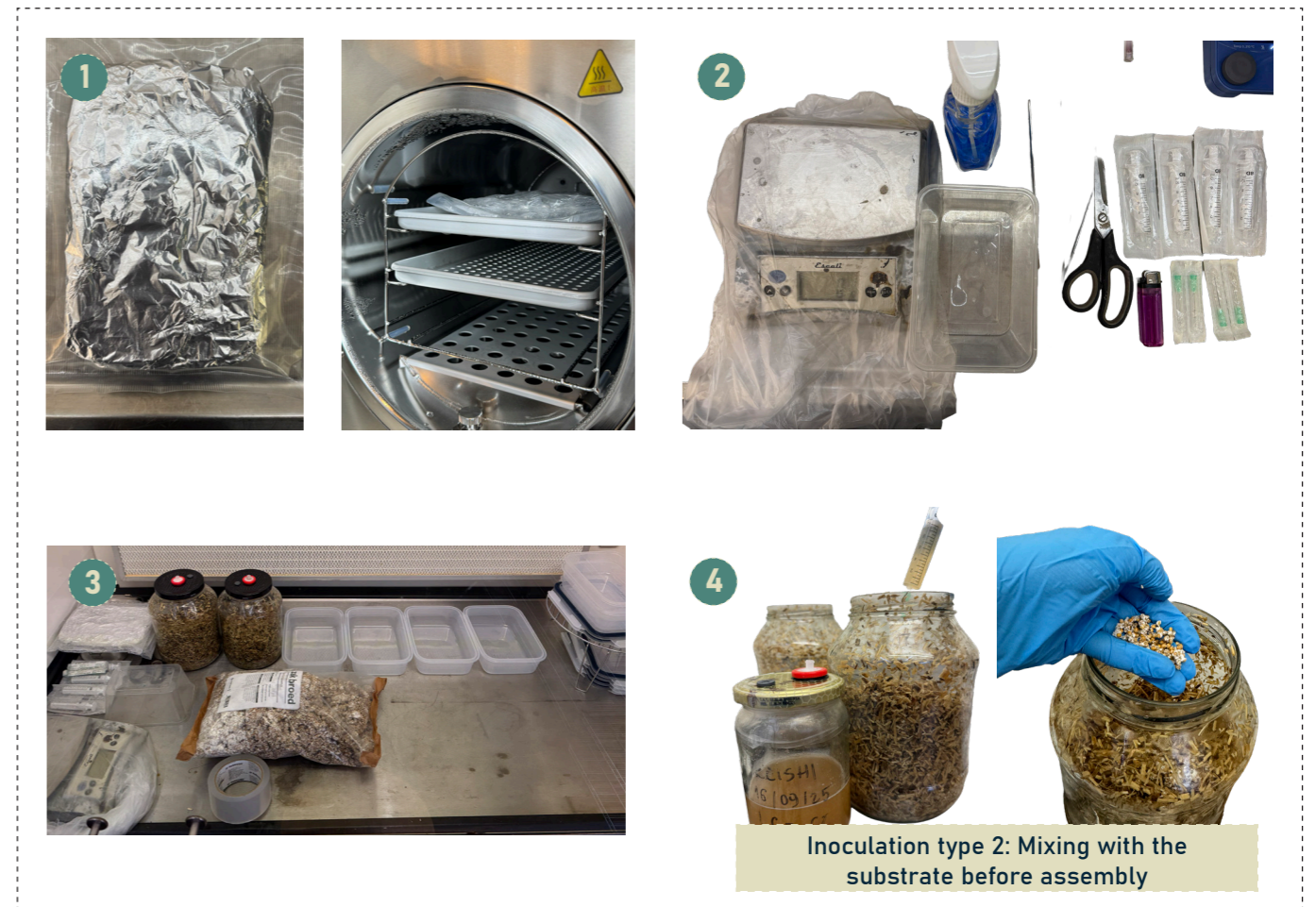
Figure 58: (1) Autoclave for WBM; (2&3) Equipments and setup; (3) Inoculation with Liquid culture and Grain spawn (Author)
