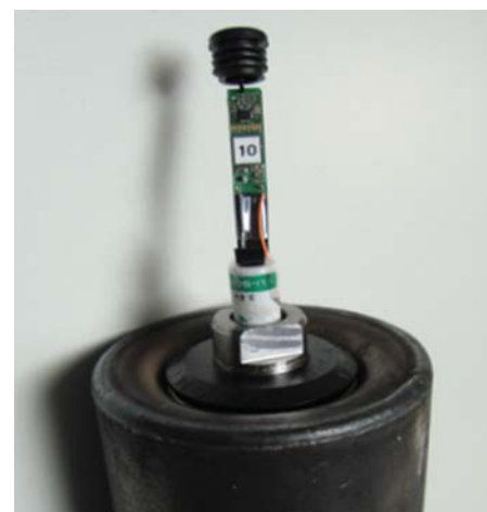
Figure 6. Idler roll with embedded sensor
