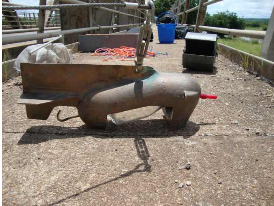
Figure B.23 D-I suspended sediment sampler
