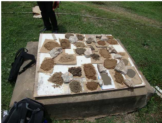
Figure B.35 Air-drying of the riverbed and riverbank samples
