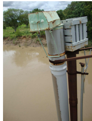
Figure B.4 Automatic water level recorder
