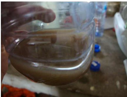
Figure B.28 The sediment is resuspended by shaking the bottle.
