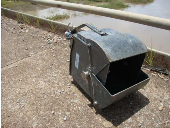
Figure B.33 Bottom sampler
