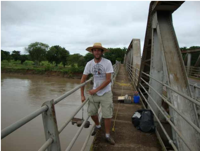
Figure B.15 Measurement of cross-section using the suspended sediment sampling device.
