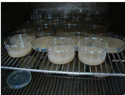
Figure B.31 The pyrex discs are dried in the oven for 3 hours at 110°C
