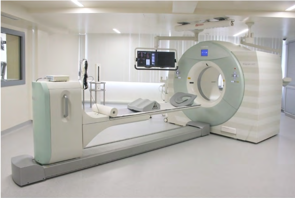
Figure 6.2: A PET/CT scanner developed by Siemens Healthcare. The frontal part of the gantry features a CT scanner, while the rear part contains a PET scanner.
