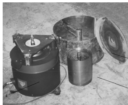
Figure 5. Coaxial cylinder tribometer developed from Kaplan (2001).
