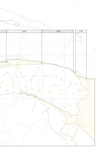
Land reclamation and the construction of sea dikes took place at different times over the entire dike section. As a result, the primary sea dikes consist of dike sections of different ages .Dike improvement in the 1970s made the dike profile uniform over the entire stretch. The palimpsest of the land is still recognizable in the form of roads and terp villages.This map shows the construction year of the sea dikes and the yellow part is the young polders.
