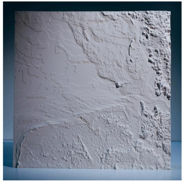
Model of the Dutch, German and Danish Waddensea, horizontal scale 1:750.000, vertical scale 1:7500 (model size 500 x 500mm). Photo: Keyan Tang, 2021.
