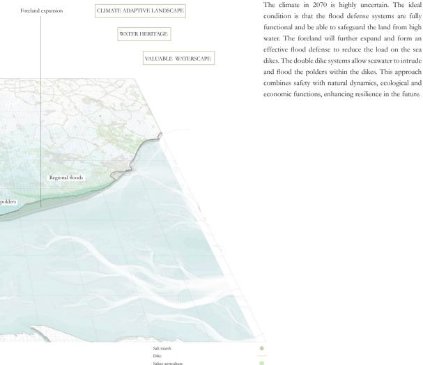
condition is that the flood defense systems are fully functional and be able to safeguard the land from high water. The foreland will further expand and form an effective flood defense to reduce the load on the sea dikes. The double dike systems allow seawater to intrude and flood the polders within the dikes. This approach combines safety with natural dynamics, ecological and economic functions, enhancing resilience in the future.
