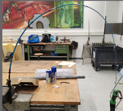
Figure 24: carbon fibre rod suspending torch.
