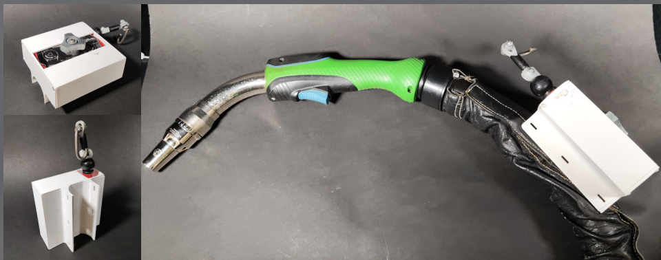
Figure 34: ExoTether. A tool balancer in a 3D printed casing that attached to the 8XE through zip-ties.
