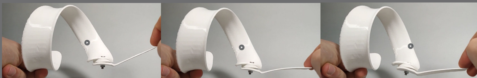
Figure 21: Helix brace - Can deflect inwards This brace was then integrated in a MIG welding glove. The helix was glued to the inside of the glove, whilst the spring was supporting the under- outside of the glove. Both parts were connected through a rotating pin.
