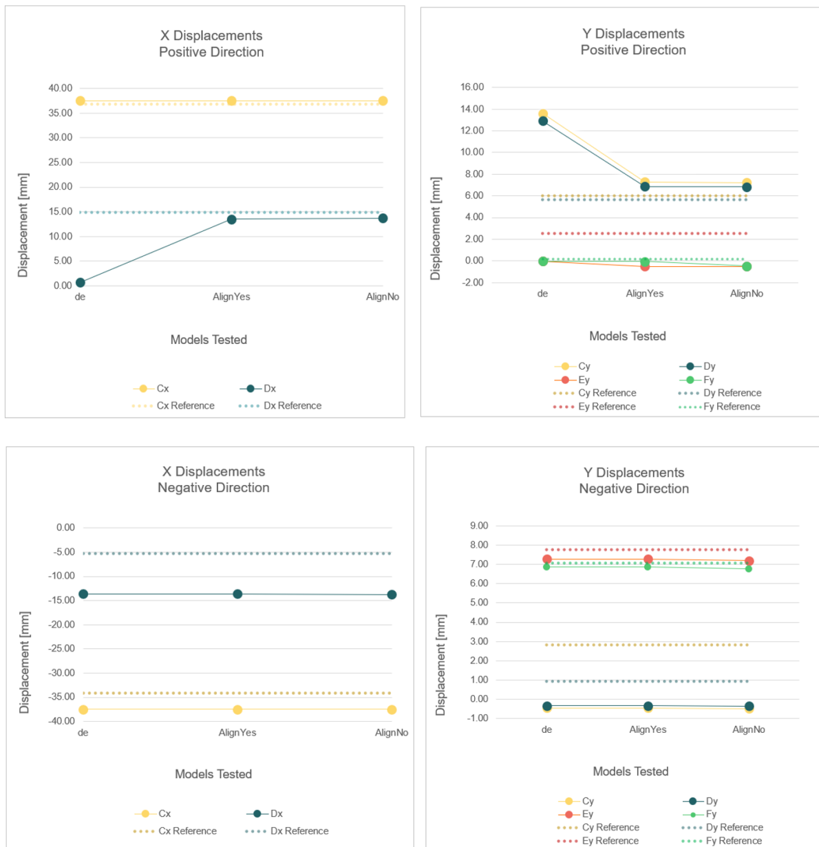
Figure C.7: The displacements both in X and Y direction of the reference points. As it can be clearly seen from the graphs, the façade response in the positive displacement recreated better the experimental behaviour compared to the negative one. A possible area of improvement is the horizontal movement of Point D.
