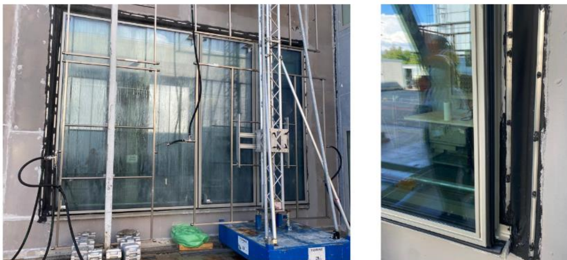
Figure 7.2: The left figure presents the implementation of water-tightness testing where water is sprayed over the curtain wall unit under testing through a grid of nozzles. The figure to the right presents the connection of the mock-up to the testing facility. During the testing it is reassured that no leakage occurs unless it penetrates through the curtain wall unit itself (Source: Permasteelisa).
