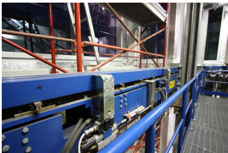
Figure 4.2: The seismic beam used for the seismic performance tests as seen from the interior of the Chamber. To the right of the picture the interesting feature of the seismic beam is visible, allowing the seismic beam to make a turn of 90.0 degrees. This feature which makes the testing of the corner of two storefronts of a building possible, was not utilised in the case study examined during this study (Source: Permasteelisa).
