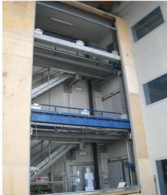
Figure 4.1: Chamber 1. The seismic and weather performance testing facility of Permasteelisa is presented. The seismic beam of the test set up can be noticed in blue (Source: Permasteelisa).
