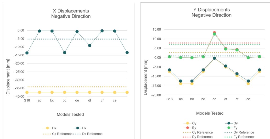
Figure D.11: The numerical values of the DIANA model for the previous scenarios tested are now accompanied by the new series of scenarios (de, df, cf and ce). The diagrams of the upper row describe the curtain wall reaction to the positive displacement application, whereas the ones of the lower row of the opposite direction.
