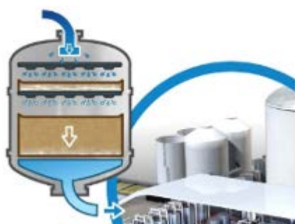
Figure 5: Cation ion exchange softener (Evides Industriewater).
