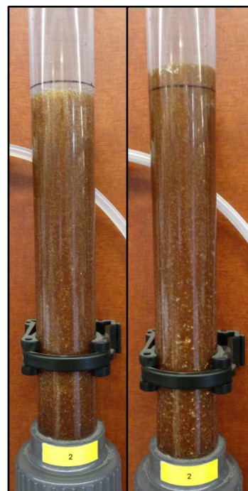
Figure 52: Gas formation in the bed during the loading of the resin.
