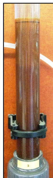
Figure 58: Deposit formation in the top of the bed.
