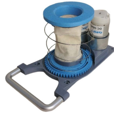
Fig. 2. General view of the BerryTwist gripper mechanism. The fabric tube is visible in the center of the picture, enclosed between the two blue rings. The upper ring is free to move as it is connected to the base only via the spring used for transferring the twisting motion. The two motors actuating the system are on the back.
