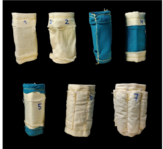
Fig. 5. Seven tubes utilized for testing blackberries. Cheesecloth tubes are depicted in white, while spandex tubes are shown in blue. Tube 7, shown on the right, is identical to Tube 6 on the left but reversed inside out.
