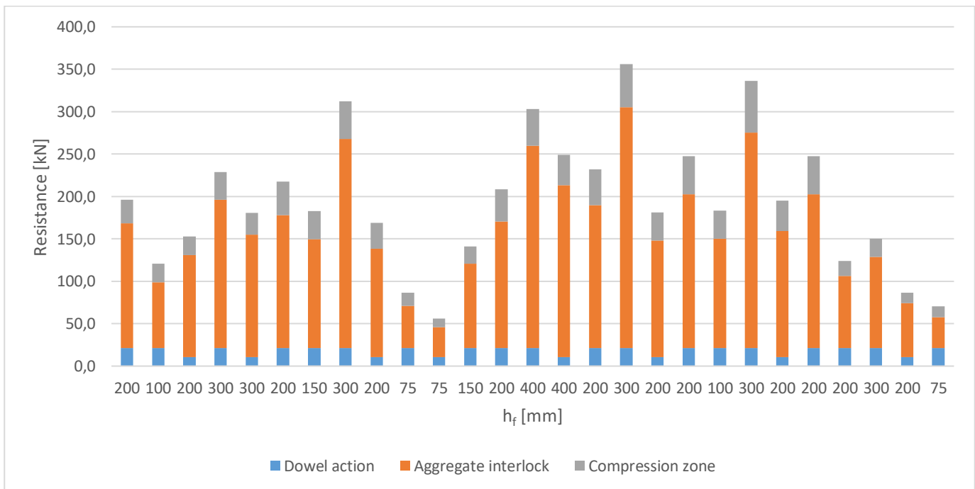
Figure 20: Overall results plates with holes in terms of flange thickness
