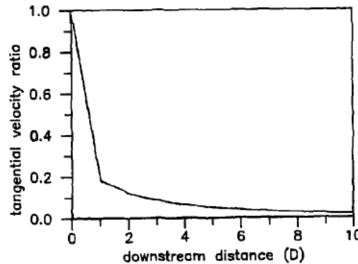
Figure 2-4: Swirl decay as a function of downstream distance, source: [43]
