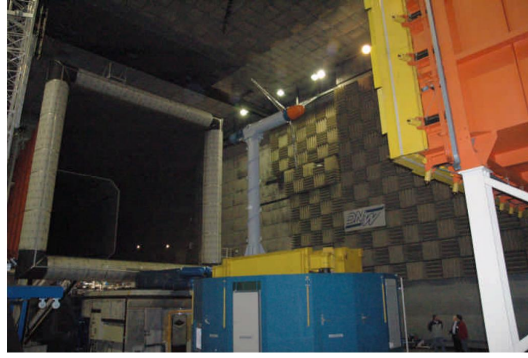
Figure 5-6: MEXICO rotor in the LLF on the six component balance
