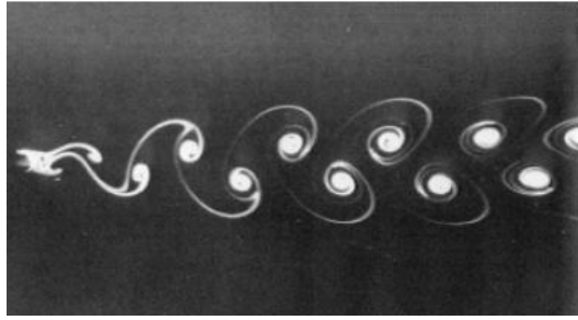
Figure 3-2: Von Karman vortex sheet behind a cylinder in uniform flow at Re = 300 , source: [7]
