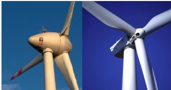
Figure 6-6: Difference in hub design of Enercon and GE turbines
