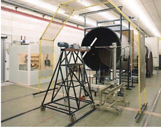
Figure 5-1: Open jet wind tunnel and model rotor, Source: [32]
