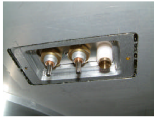
(b) The battery charge stud and activation switches, mounted on the bottom honeycomb panel of SSETI Express [6]
