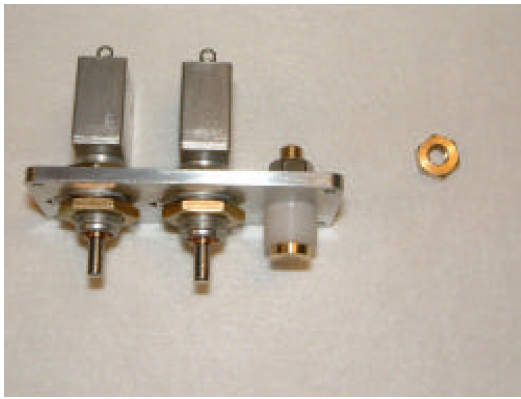
(a) The battery charge stud and activation switches, as a standalone module [6]
