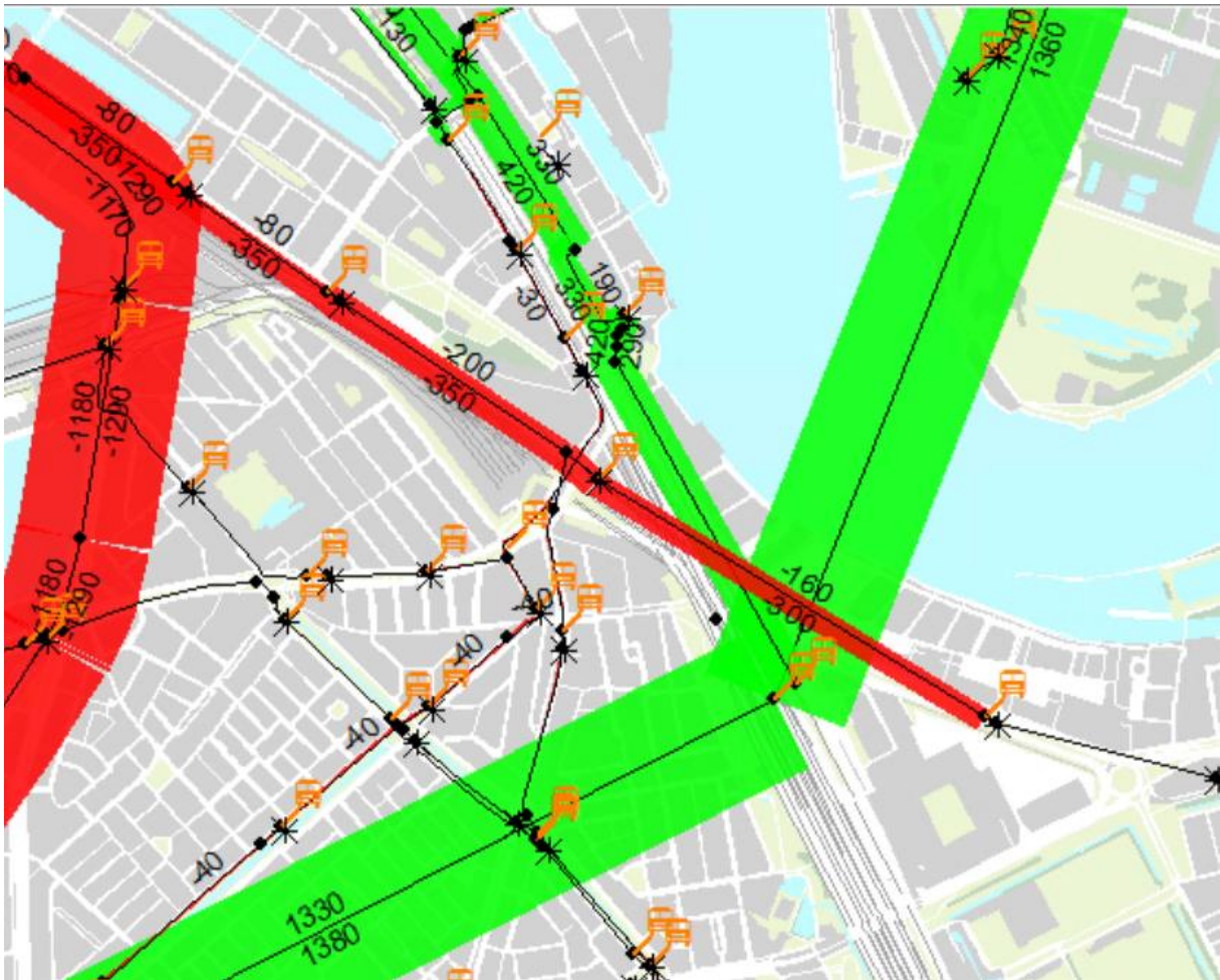
Figure 19 Bandwidth visualization of difference in travelers between variant and reference over the links in the network for a traffic assignment without elasticities (OV-Lite) Apparently the extension of bus 32 creating a bus connection between station Zuid and station Stadionpark, which gives access to the new rail tangent, provides a shorter route to 290 (from Stadionpark) and 420 (to Stadionpark) travelers.
