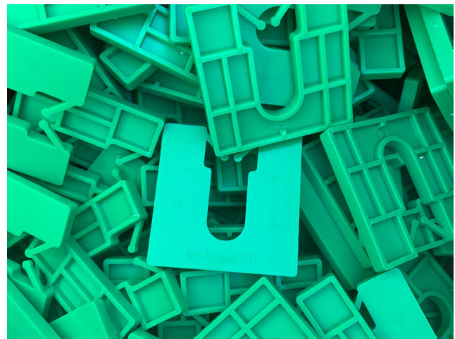
Figure 6.8 Filler plates (Picture taken by author)
