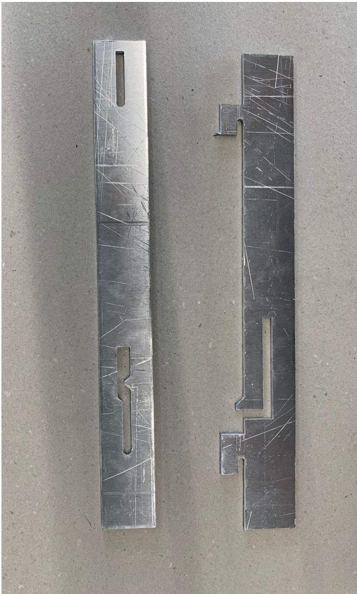
Figure 8.24 Snap fit test plates. Left: Omega front flange. Right: Cassette panel side flange. (Pictures taken by author)
