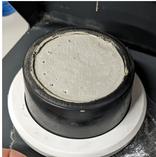
Figure 6.2: Picture of P/0.8 sample after the setting time test
