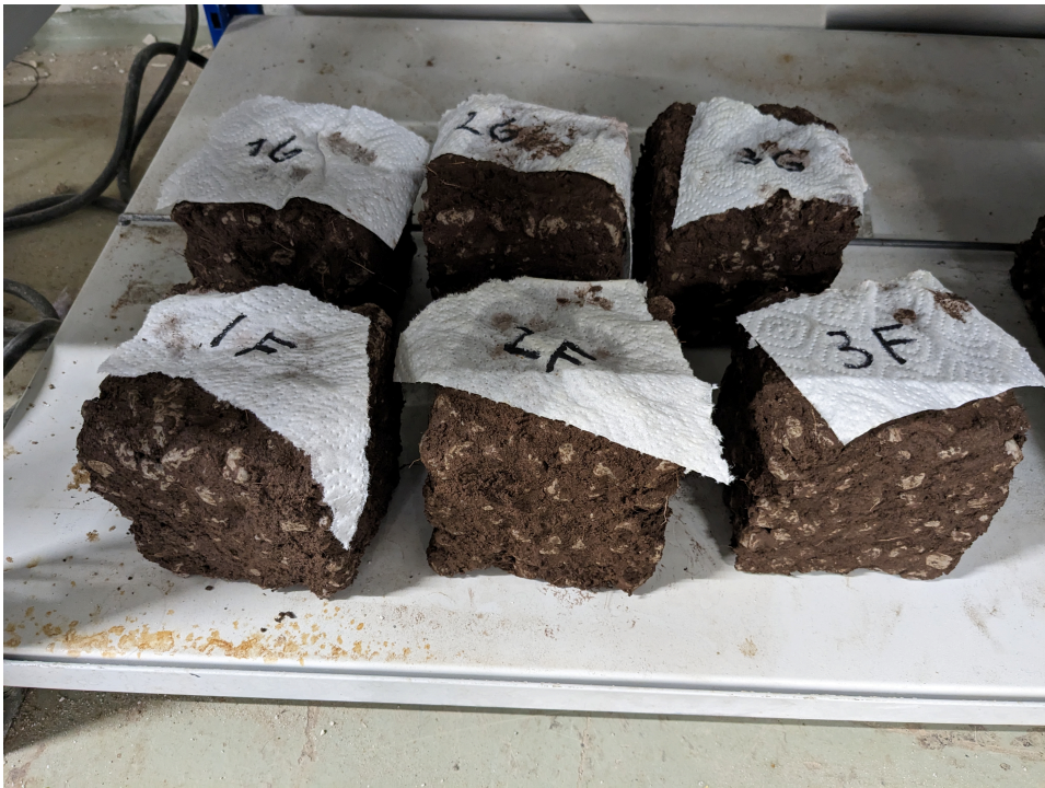
Figure 6.33: Images of the cubes with soil before the first experiment is conducted
