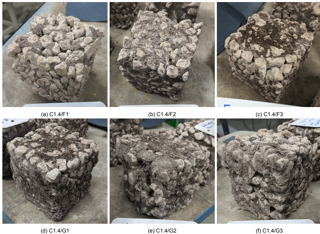
Figure 6.34: Images of the cubes with soil after immersion in water to determine the maximum water absorption capacity
