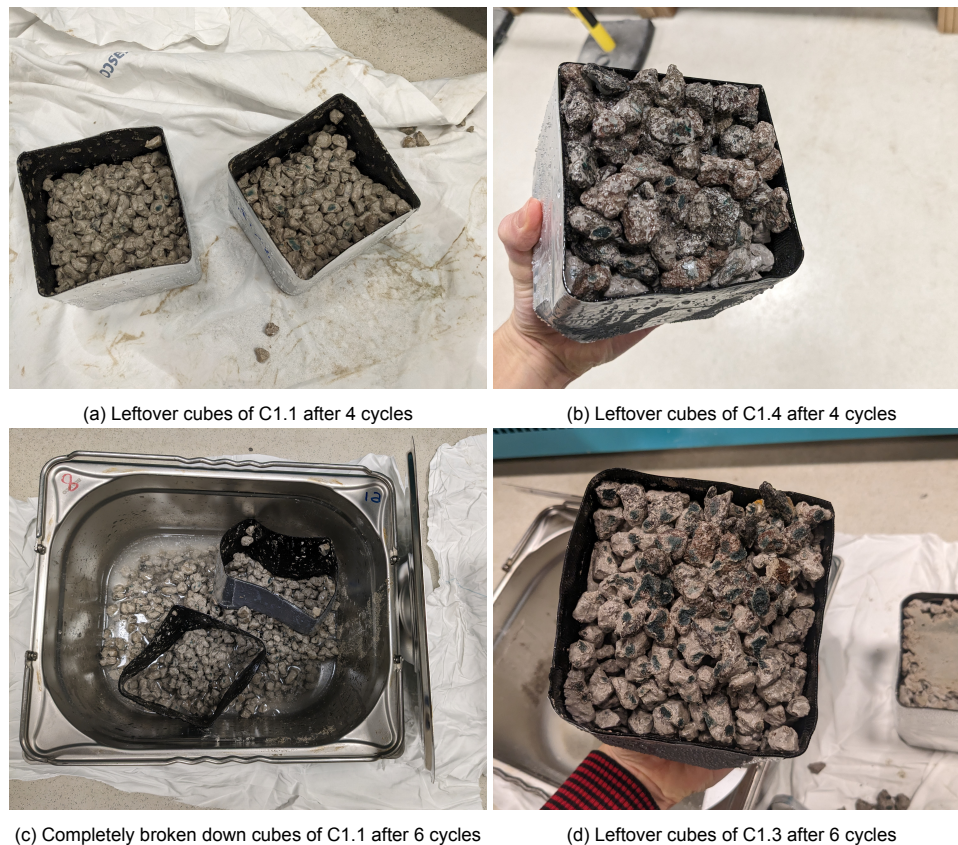
Figure 6.25: Images of failure due to FT cycles
