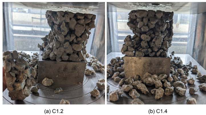
Figure 6.13: Failure pattern of compressive strength testing at 28-day curing age
