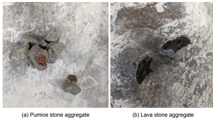
Figure 6.14: Failure of the aggregate
