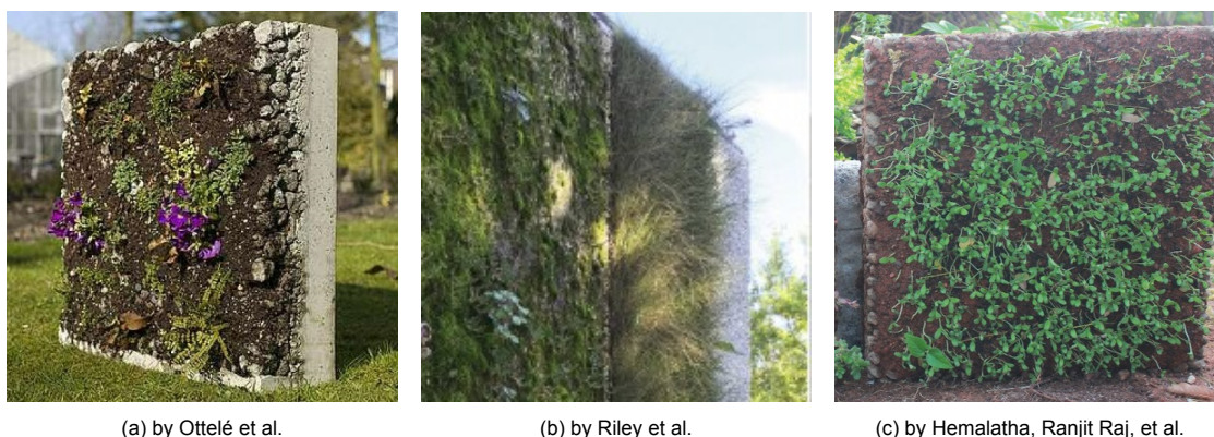
Figure 2.2: Pictures of test samples of vegetated pervious concrete tested in previous research
