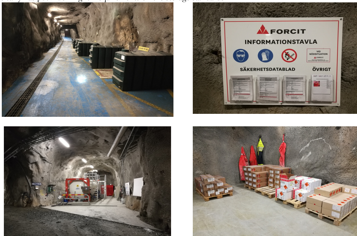
FIGURE 16: IMPRESSIONS FROM, CLOCKWISE FROM TOP LEFT; WATER BUFFERS IN THE MAGAZINE BETWEEN STORAGE SECTIONS IN TARA, PERMITS AND INSTRUCTION MANUALS IN KANKBERG, EMULSION STORAGE IN KANKBERG AND ORDERLY PRIMER STORAGE PRIOR TO CHECKOUT IN KANKBERG
