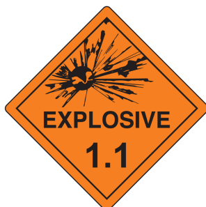
FIGURE 8: EXAMPLE OF SIGN TO BE USED ON PRODUCTS WITH A MASS EXPLOSION RISK
