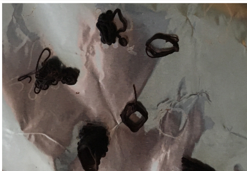
Figure 4 - Cacao shell flour with K-Carrageenan and sodium silicate liquid
