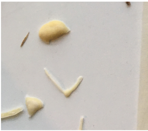
Figure 2 - Sagged prints, no printing lines visible anymore
