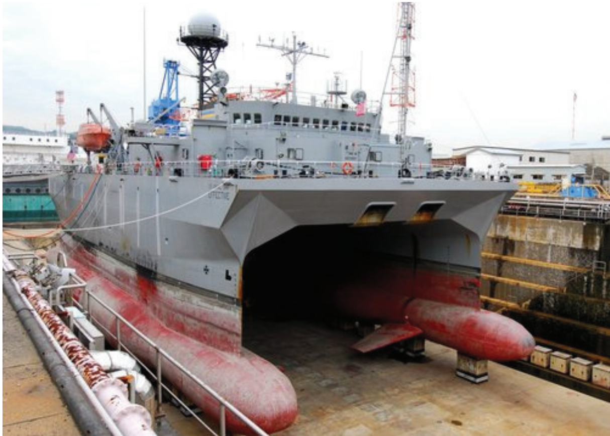
FIGURE 2-4: SWATH DESIGN WITH FINS SOURCE: MCKEESON.US
