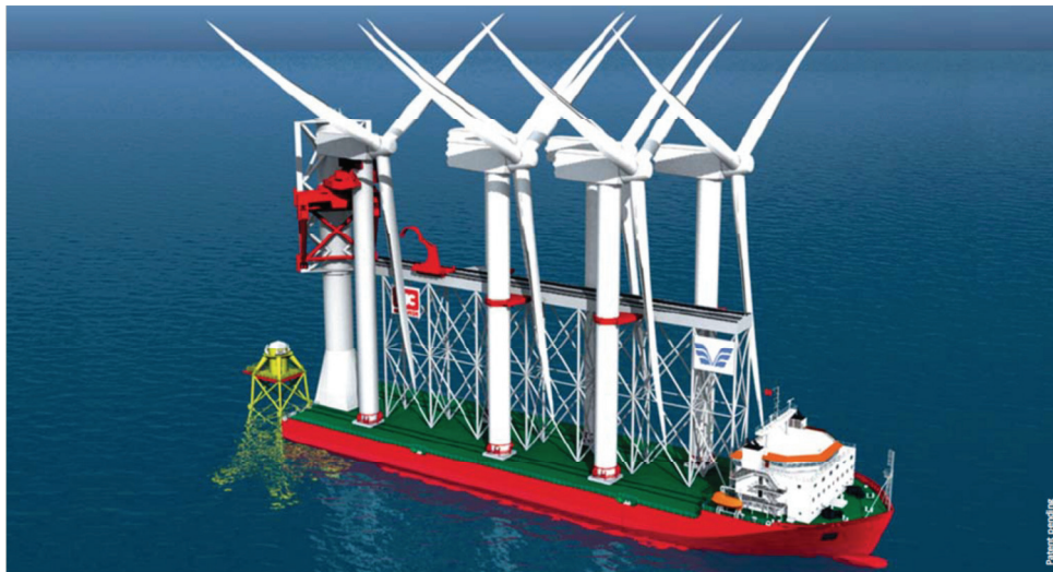
FIGURE 2-3: MONOHULL WITH COMPLEX INSTALLATION SYSTEM SOURCE: IHC.
