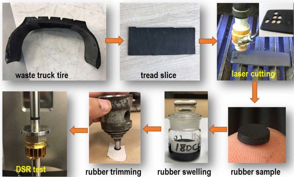
Fig. 2. Preparation of cylindrical rubber samples for DSR tests.
