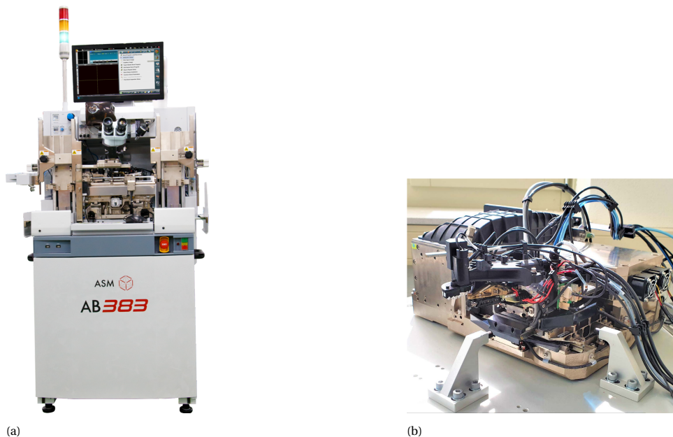
Figure 10.14: (a) ASMPT wire bonder whose motion stage was utilized in this work. (b) Isolated XYZ-motion platform of the wire bonder.
