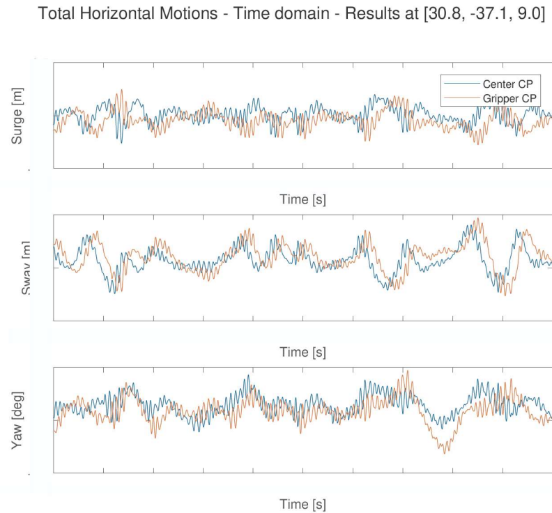
Figure 5.2: Total motions in the horizontal plane during 3h time domain simulation in H_s = 1.5 m, wavedir. = 135 deg and T_p = 8 s; results obtained at t = ***
