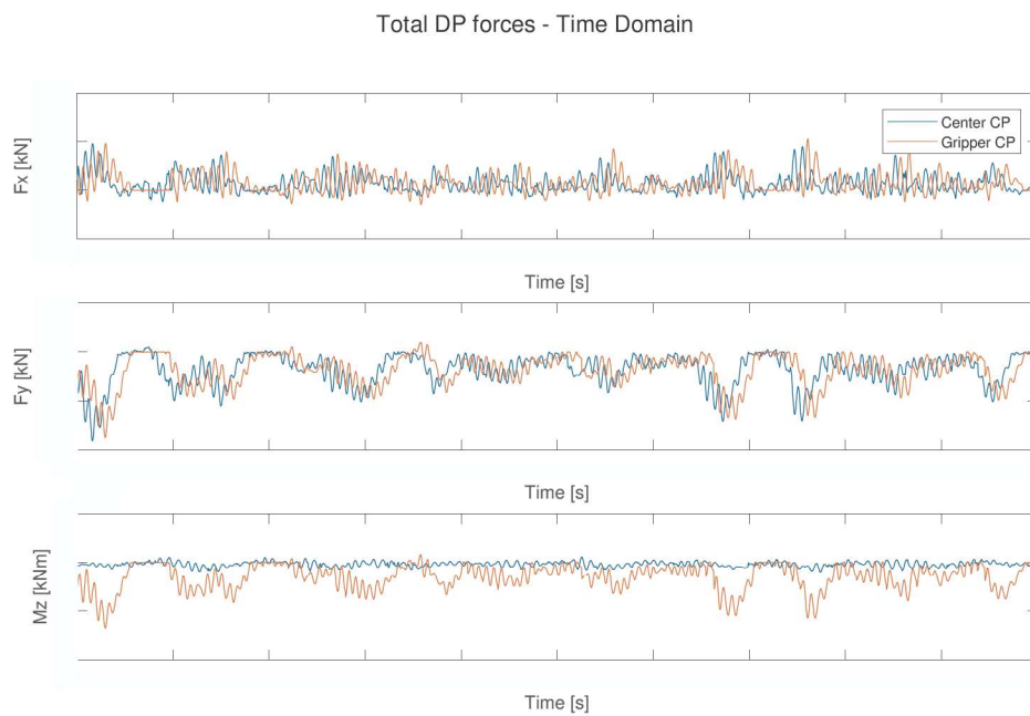
Figure D.4: DP Forces during 1h time domain simulation in H_s = 1.0\text{m} , \text{wavedir.} = 135\text{ deg} and T_p = 8\text{s} ; results obtained at t =
