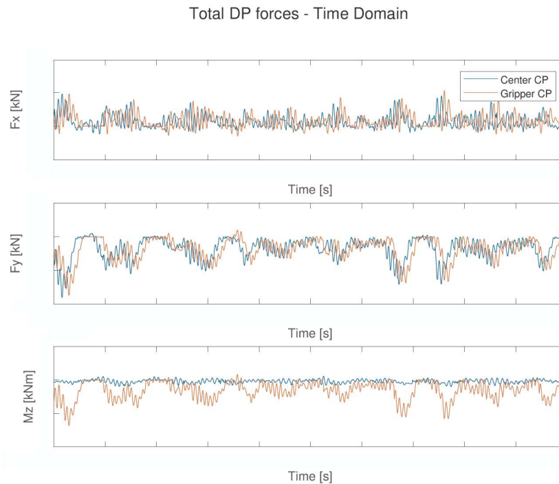
Figure 6.10: DP Forces during 1h time domain simulation in H_s = 1.0\text{m} , wavedir. = 135 deg and T_p = 8\text{s} ; results obtained at t = [2000\ 3000]
