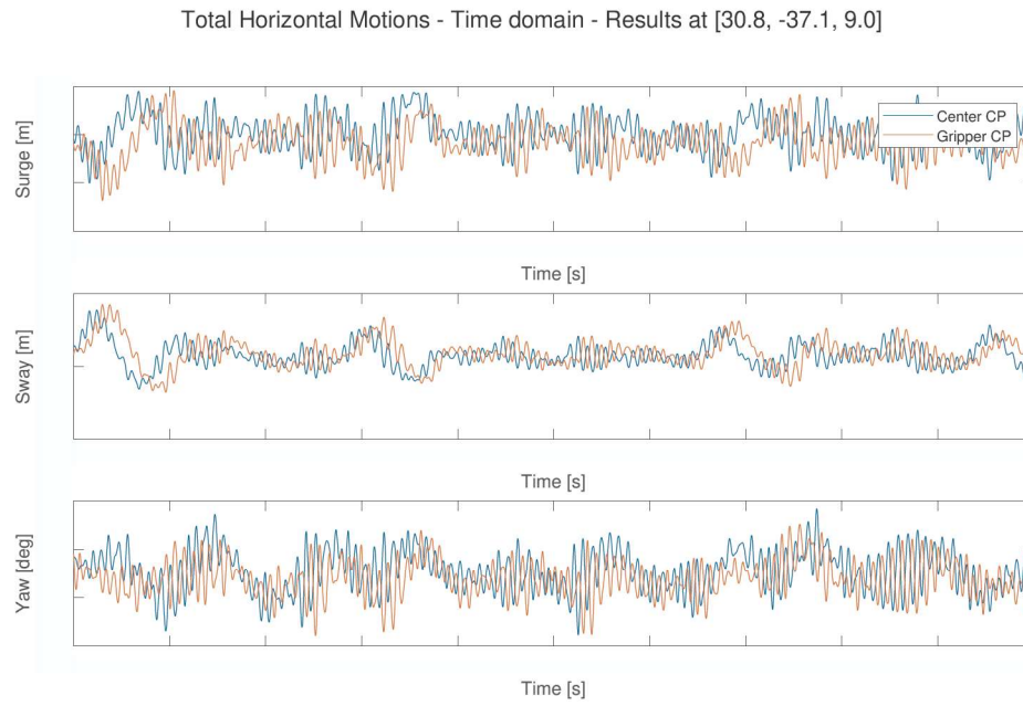
Figure D.2: Total motions in the horizontal plane during 1h time domain simulation in H_s = 1.0\text{m} , \text{wavedir.} = 135\text{ deg} and T_p = 8\text{s} ; results obtained at t =
