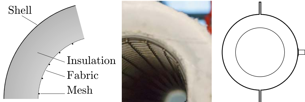
Fig. 1 Schematic representation of a portion of the sample cross-section with components indicated (left), sample 18-1H-1 before adhesion of the connectors (middle), and schematic representation of a sample during testing with the shell flanges vertical and a gas thermocouple mount on one side (right)
