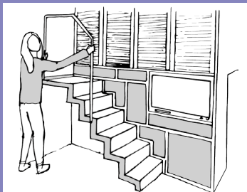
PULL-OUT STAIRS hidden - action required minimal space needed moderately comfortable
