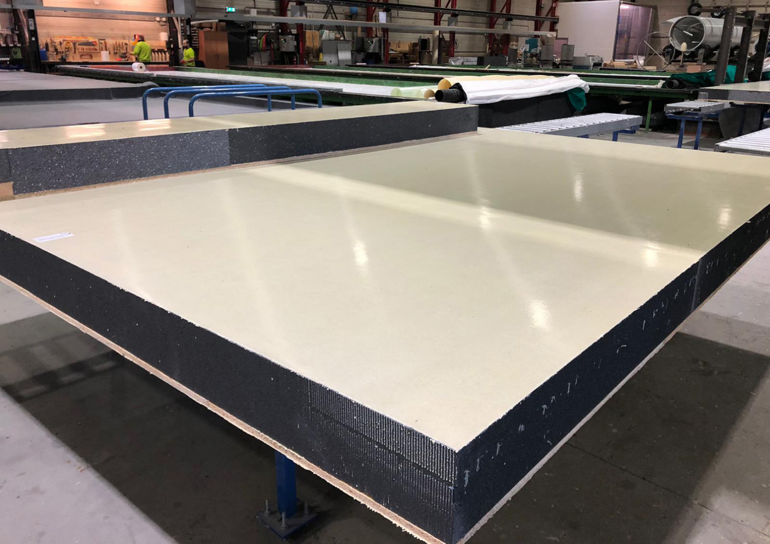
Figure 25 RC Panel without decorative finish (picture by the author)
