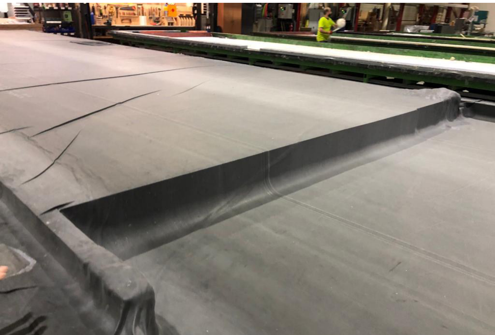
Figure 24 RC Panels Factory - Vacuum process (picture by the author)
