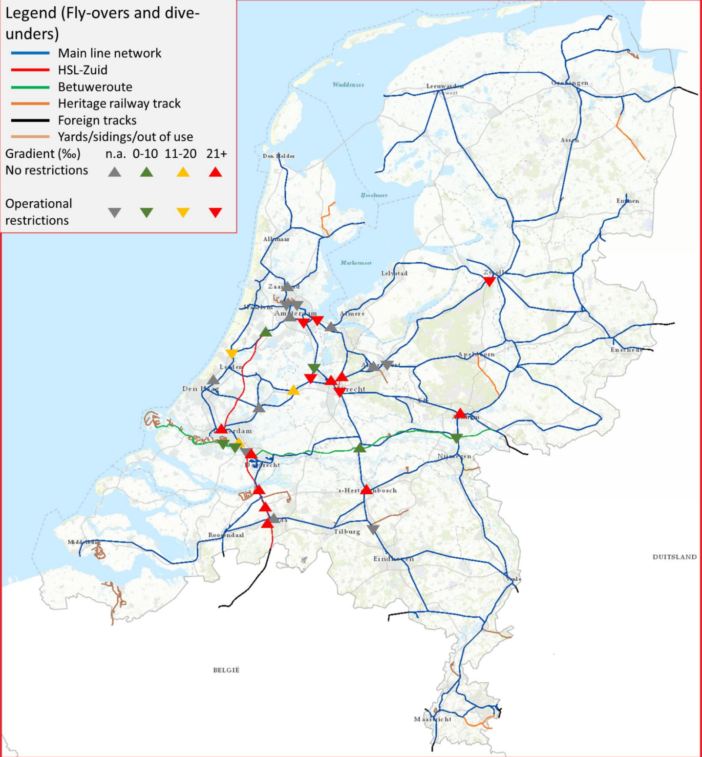
Figure 15, Gradients at fly-over and dive-unders
