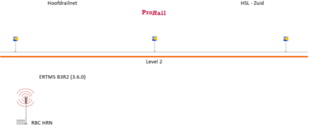
Figure 22, solution 3: RBC integration of HSL
