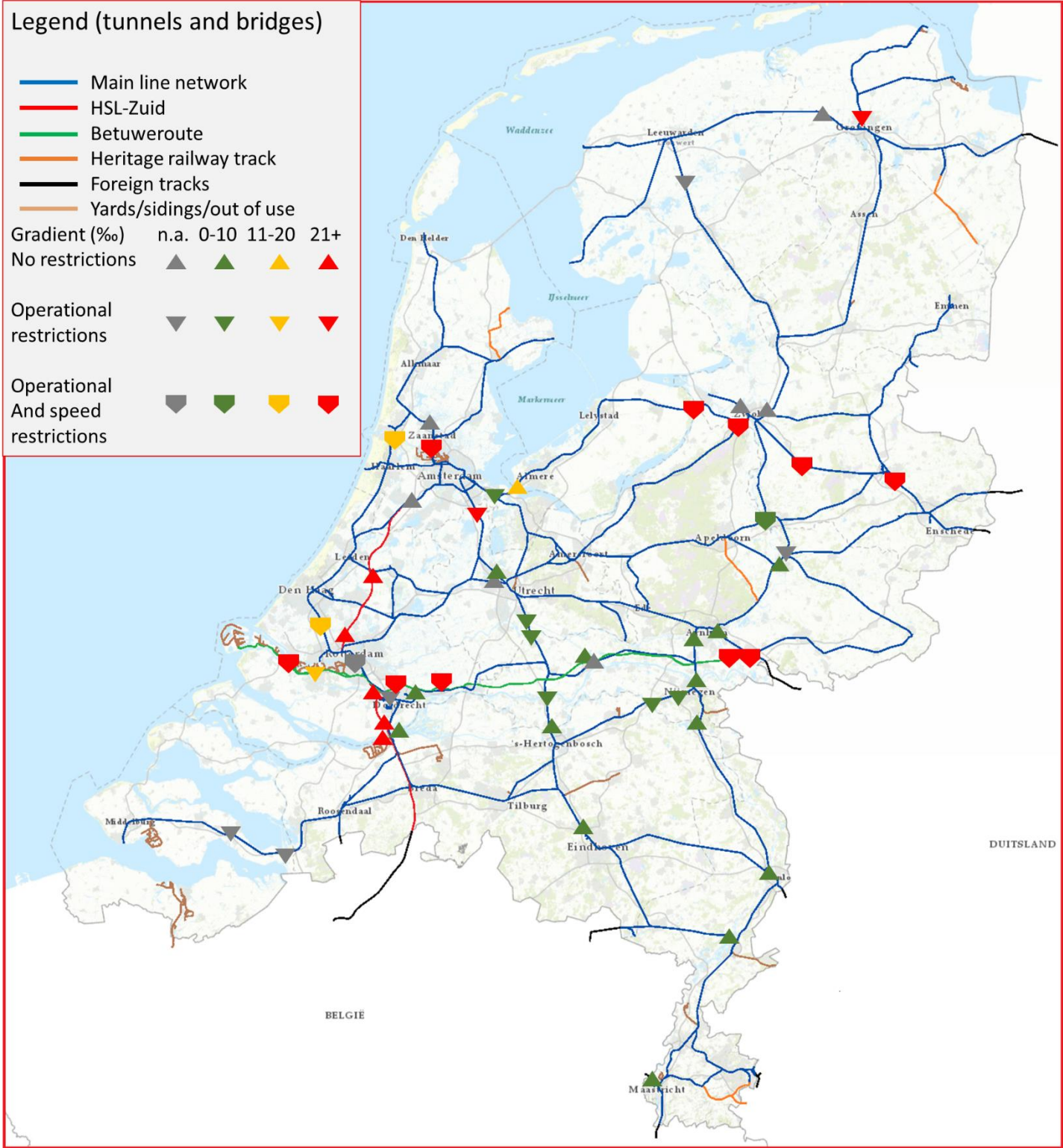
Figure 14, Gradients at tunnels and bridges
