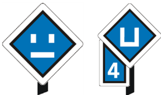
Figure 10 Signs indicating 'power off' left and 'power on' right'
