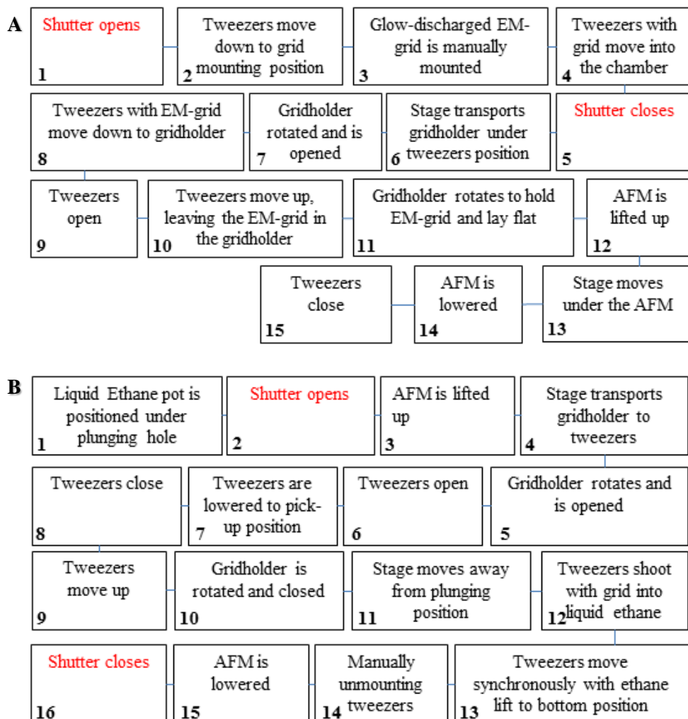
Figure 5.3: Flowcharts summarizing the different steps necessary to place an EM-grid in the gridholder for (A) liquid manipulation experiments with the hollow AFM cantilever or for (B) pick-up of the EM-grid after dispensing and plunge freezing in liquid ethane. The following steps are automated by the software designed by Daniel Torres-Gonzalez. (A) Steps 6-14 are automated. (B) Steps 3-12 are automated. The steps involving the shutter are coloured red, because the shutter is not installed yet and these steps are not as yet executed.
