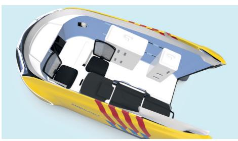
EXTERIOR STORAGE increases the efficiency of THE INTERIOR features modular storage units the workflow, allowing for quick and easy access and chairs that can be positioned anywhere. This way the interior can be adapted to any situation.
