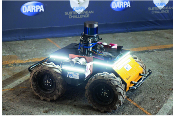
Figure 1-1: The husky platform participating in DARPA's SubT Challenge. The contest demonstrates the requirement of improving safety and efficiency for underground search-and-rescue missions, from [23]
