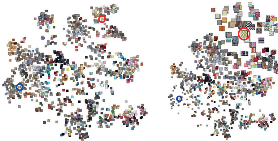
Figure 4.3: Original embedding (left) and modified embedding using prioritized t-SNE (right). The texture circled in red was given a higher priority with W = 8 in Eq. 4.1, resulting in larger distances between images for all similar images, which are also enlarged to improve visibility. Conversely, the image circled in blue was given a low priority with W = 0.2 in Eq. 4.1, contracting similar images together.
