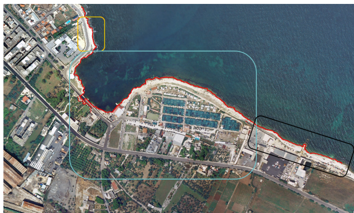
Figure 3.11.: Example of the shoreline extracted along Apulian beaches overlapped on ortho-images. The yellow box delimits the breakwater zones, the blue box marks the rocky beaches, and the black box delimits sandy beaches limits.
