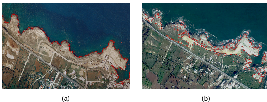
Figure 3.12.: Comparison between shoreline detected during calm and rough sea. Example of the influence of wave foam on the shoreline detection. (a): Rocky beaches shoreline extraction along the Apulian region during calm sea; (b): Rocky beaches shoreline extraction along the Apulian region during rough sea.
