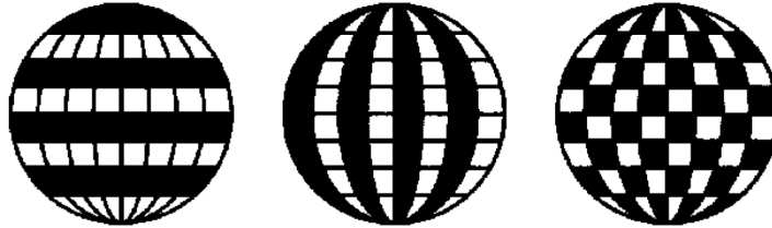
Figure 2.2: White areas are elevations above and black areas elevation below a mean spherical surface. Zonal deviations on the left ( m = 0 and n \neq 0 ), sectorial deviations in the middle ( m = n \neq 0 ) and tesseral deviations on the right ( 0 \neq m < n ) [46].
