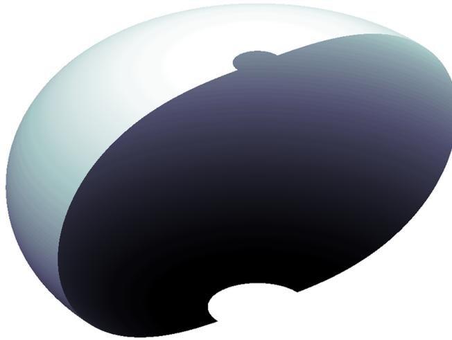
Fig. 6.11: Sectional 3D profile for the isotensoids obtained using the present method
