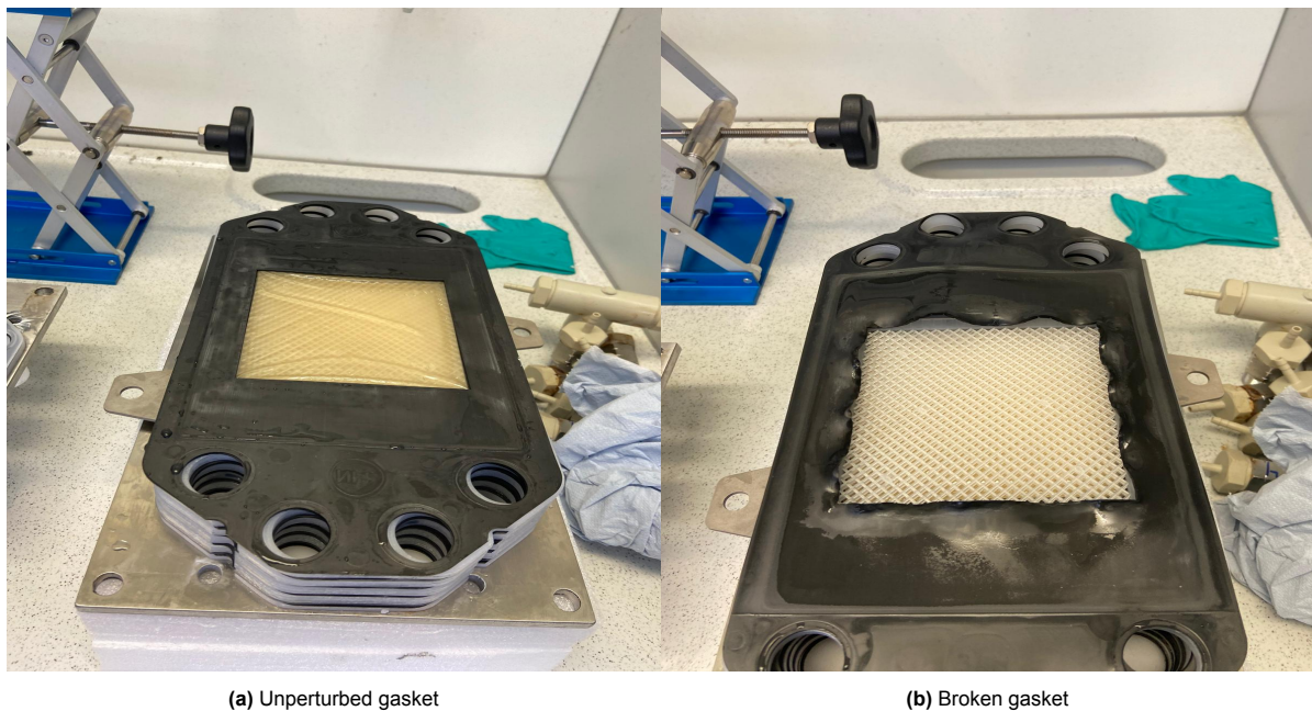
Figure 5.10: Display of working and broken EPDM gaskets
