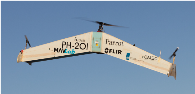
Figure 2: DelftaCopter in hover. In forward flight, the entire fuselage pitches down 90^\circ and the rotor provides the thrust as shown in Figure 1.
