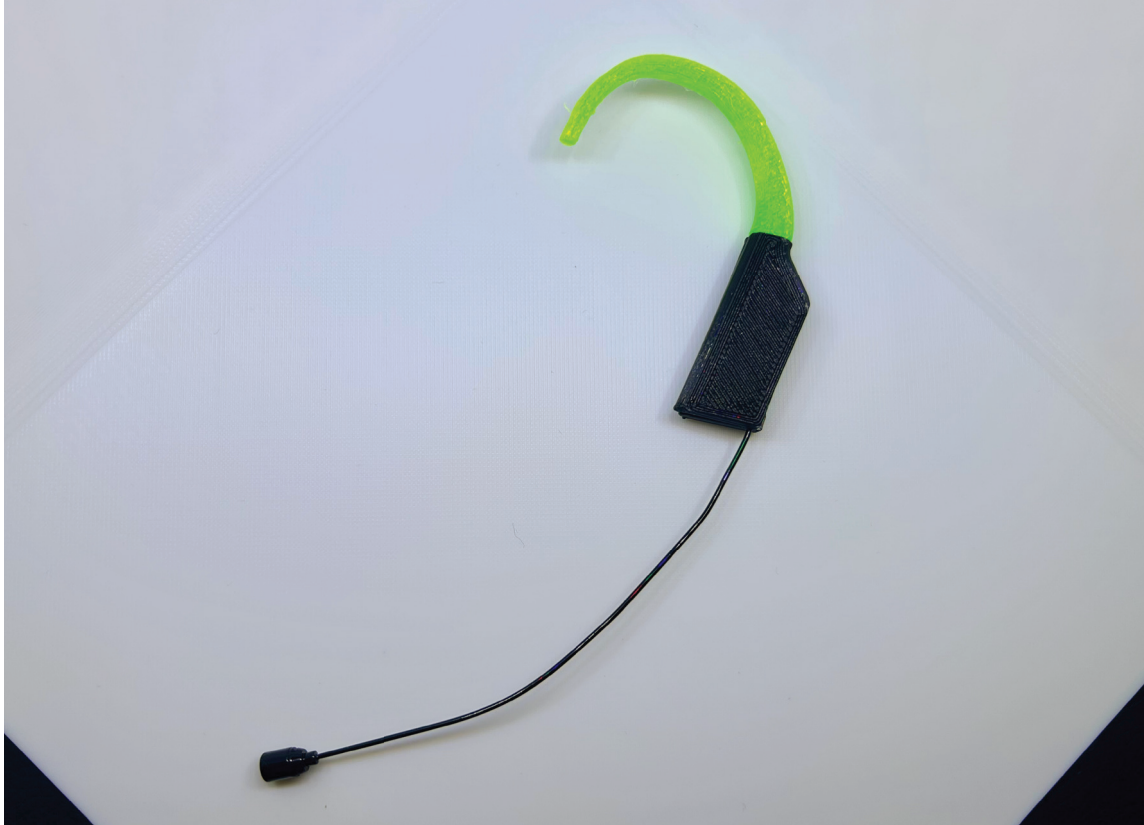
Figure 38: Prototype featuring a moldable ear hook and hard casing with microphone wire.
