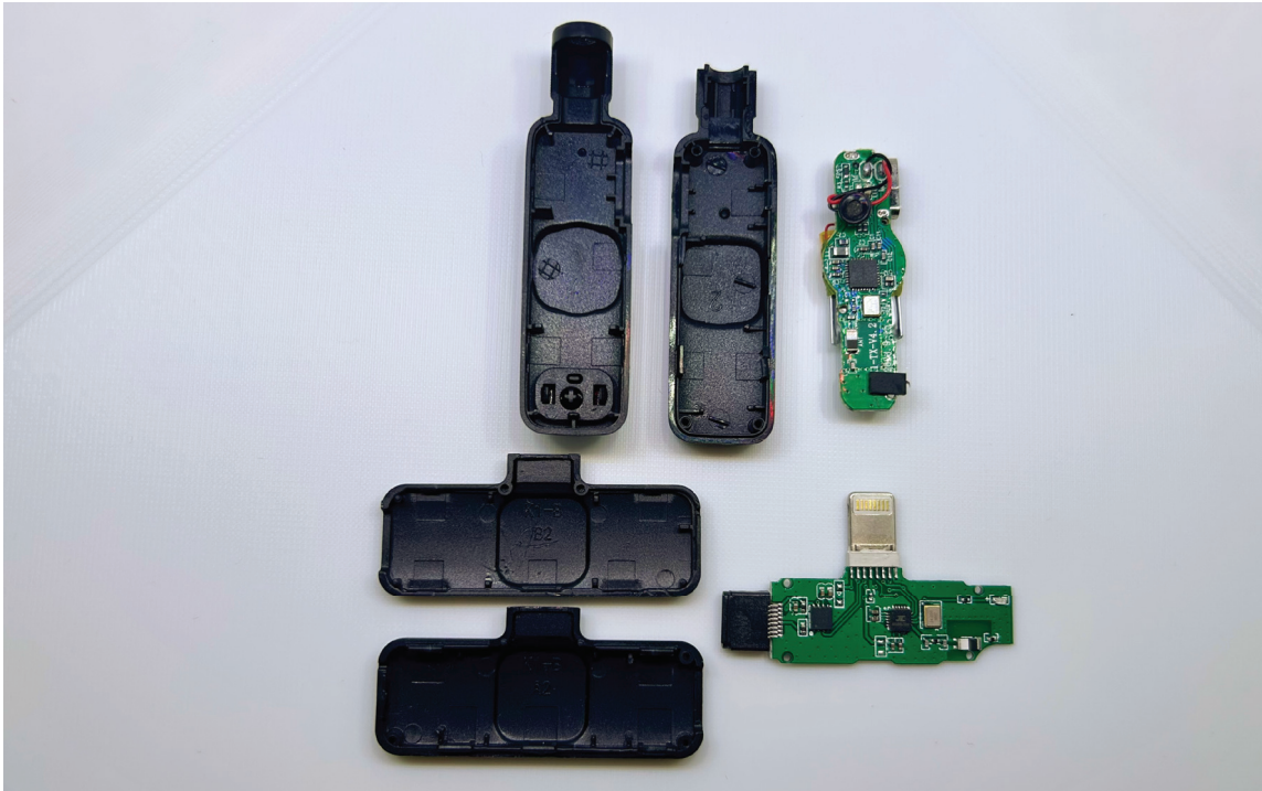
Figure 48: Disassembled view of the HUACAM Lavalier showing key internal components, including the battery, printed circuit boards, microphone, Lightning connector, and housing parts
