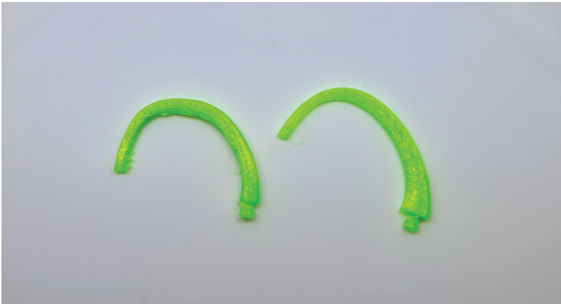
Figure 37: Prototypes of a moldable ear hook reinforced with a metal wire to change the shape
