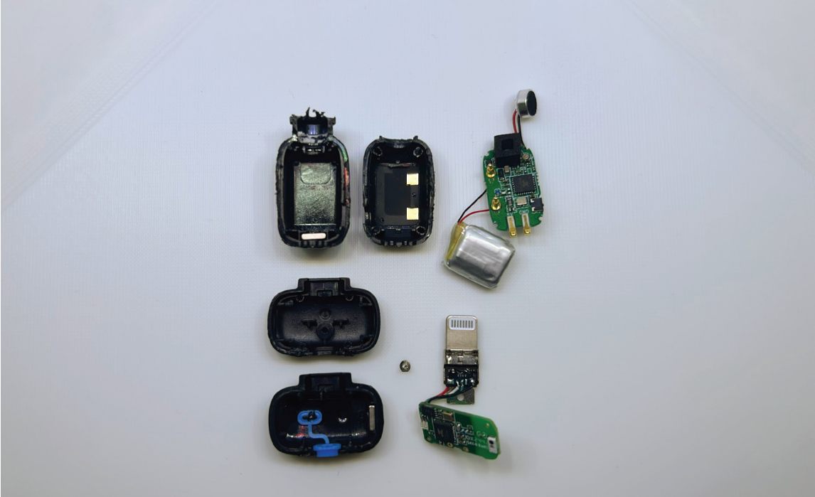
Figure 47: Disassembled view of the BOYA mini showing key internal components, including the battery, printed circuit boards, microphone, electrical contacts, Lightning connector, and housing parts
