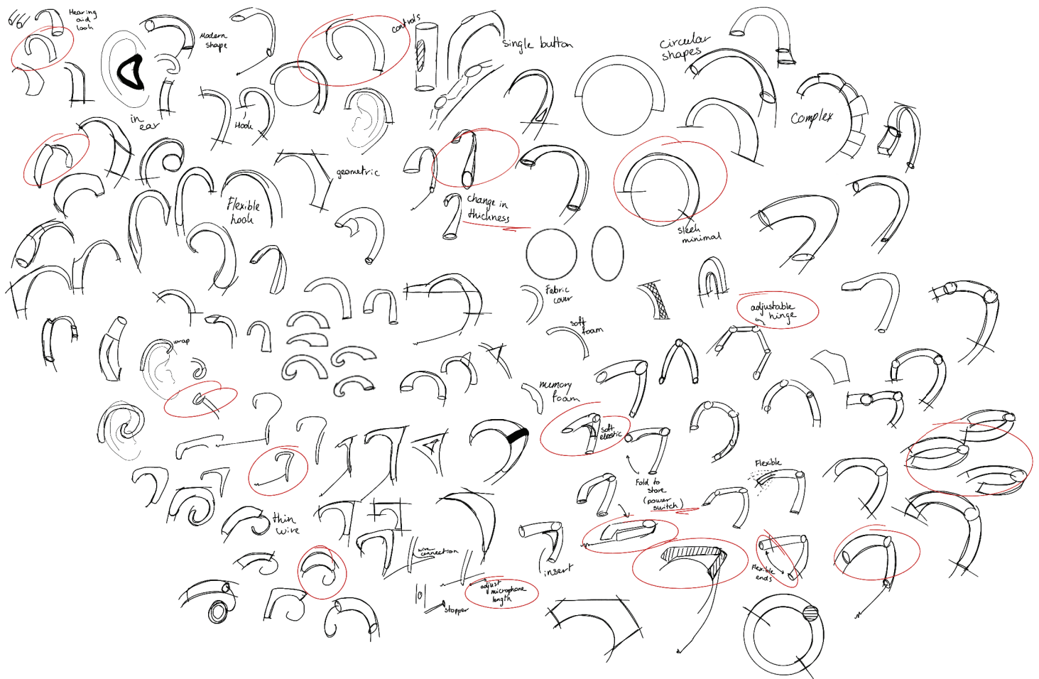
Figure 50: Figure: Exploratory sketches investigating alternative shapes to minimise product size
