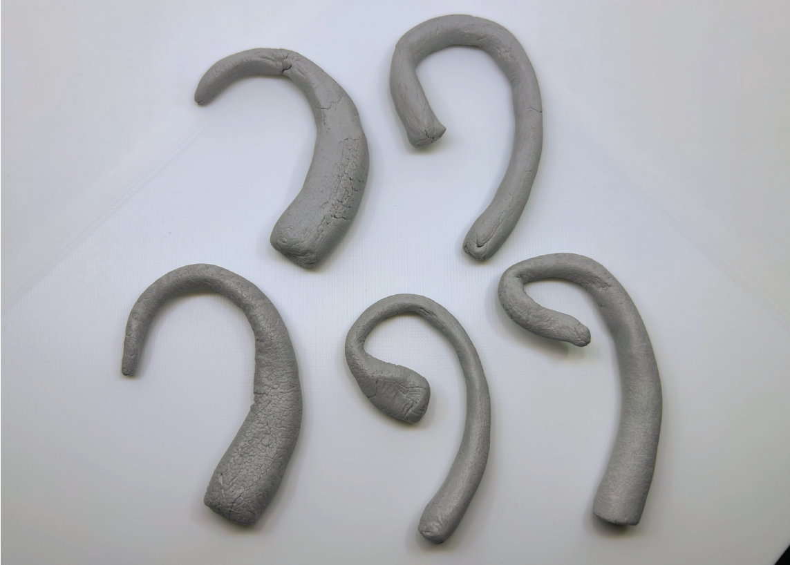
Figure 34: Various clay models exploring methods of securing the microphone body to the ear
