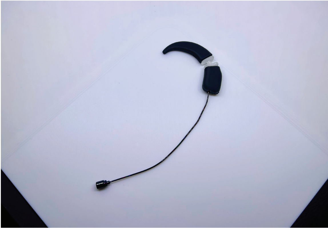
Figure 53: Final combined design of the wearable microphone. It comprises two separate bodies that contain the internal components, as well as a hinge mechanism with an internal wire for size adjustment.
