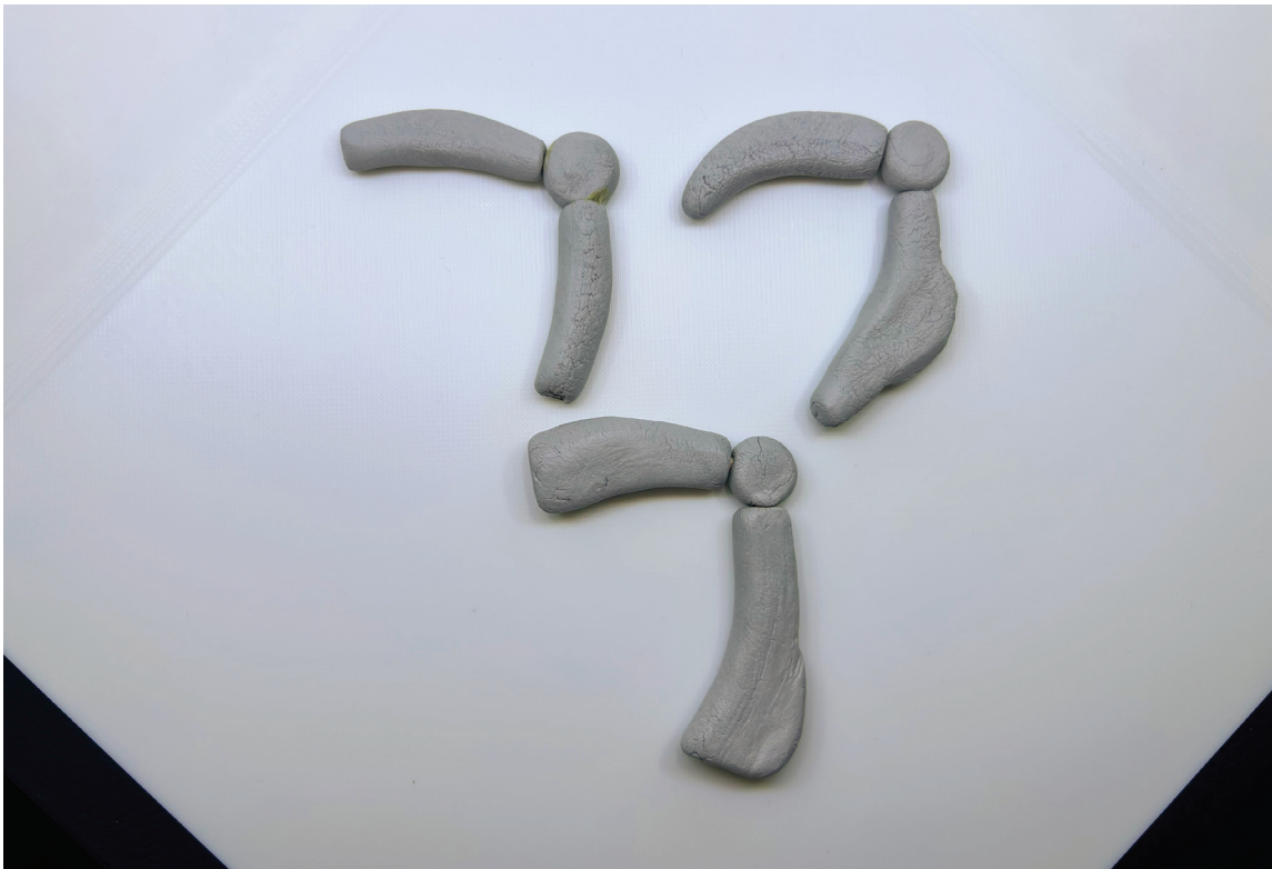
Figure 52: Clay models with a hinged structure that can be adjusted to different sizes, featuring varied body shapes to accommodate different internal component layouts
