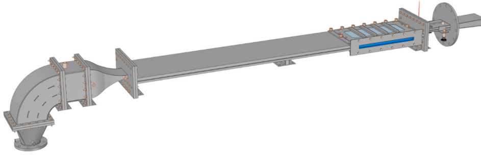
Fig. 1. 3D CAD representation of the testing section of the FTFC.
