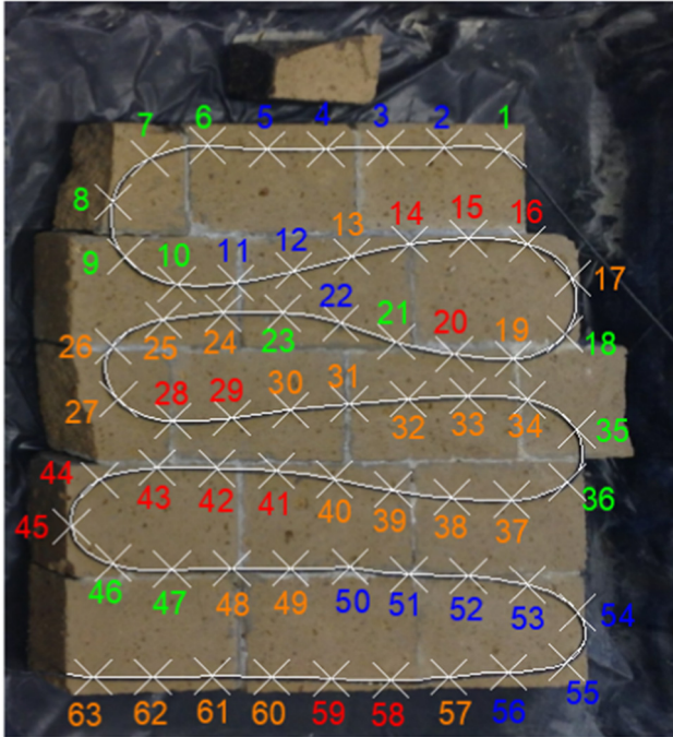
Fig. 5. Numbered measurement points (X) and temperature map. Red = hot, Orange = warm, Green = cool, Blue = cold. (For interpretation of the references to color in this figure legend, the reader is referred to the web version of this article.)
