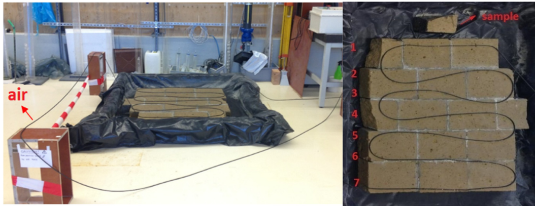
Fig. 2. Experimental setup (left) and active DTS cable layout on the tuff wall with indication of straight cable segments (right).
