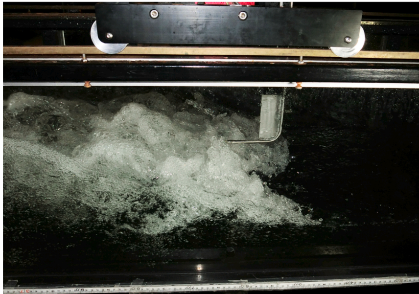
(B) Hydraulic jump for Fr_1 = 2.1 , Re = 1.97 \times 10^5 , d_1 = 0.097 m, x_1 = 1.5 m, B = 0.5 m, shutter speed: 1/500
