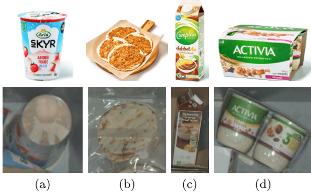
Figure 4.3: Representative ambiguity cases during automated reference-pool construction. Each column shows a SKU template image in the top row and a candidate product crop extracted from a stock-container image in the bottom row. (a) A transparent upside-down product may resemble leaked or spilled content. (b) The template and operational product appearance may differ. (c) Secondary packaging text or advertisements may be confused with a wrong product. (d) A valid package orientation may resemble opened packaging. These cases illustrate a limitation of conservative VLM-based filtering: valid normal appearances may be excluded from the reference pool when they are visually ambiguous or differ from the template appearance.
