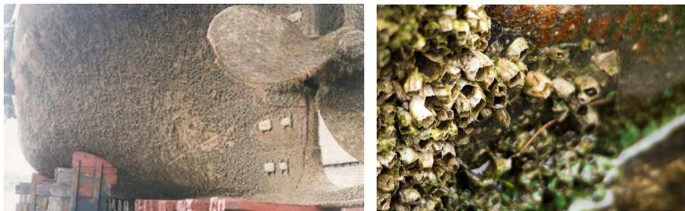
FIGURE 1.1: Two examples of biofouling: fouled ship hull (*left*)<sup>2</sup>, and fouling close-up (*right*)<sup>3</sup>.
