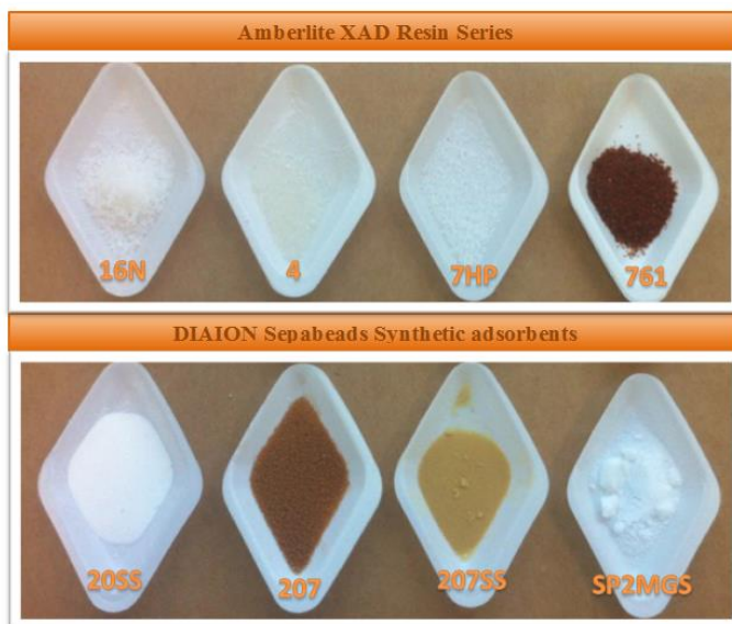
Figure 3.2 Tested synthetic adsorbents from Amberlite XAD resins and DIAION Sepabeads
