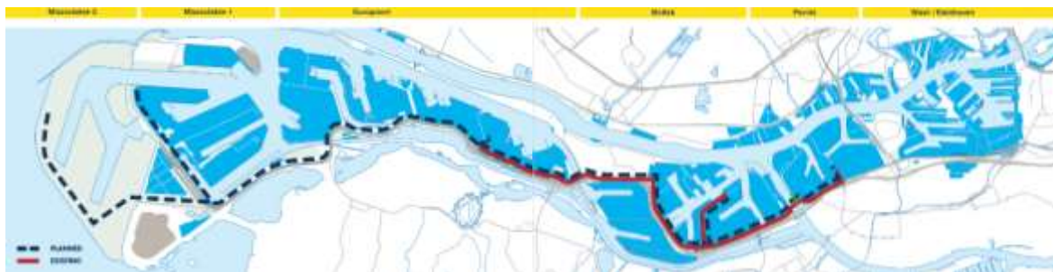
Figuur 17. MultiCore pipeline system Rotterdam
